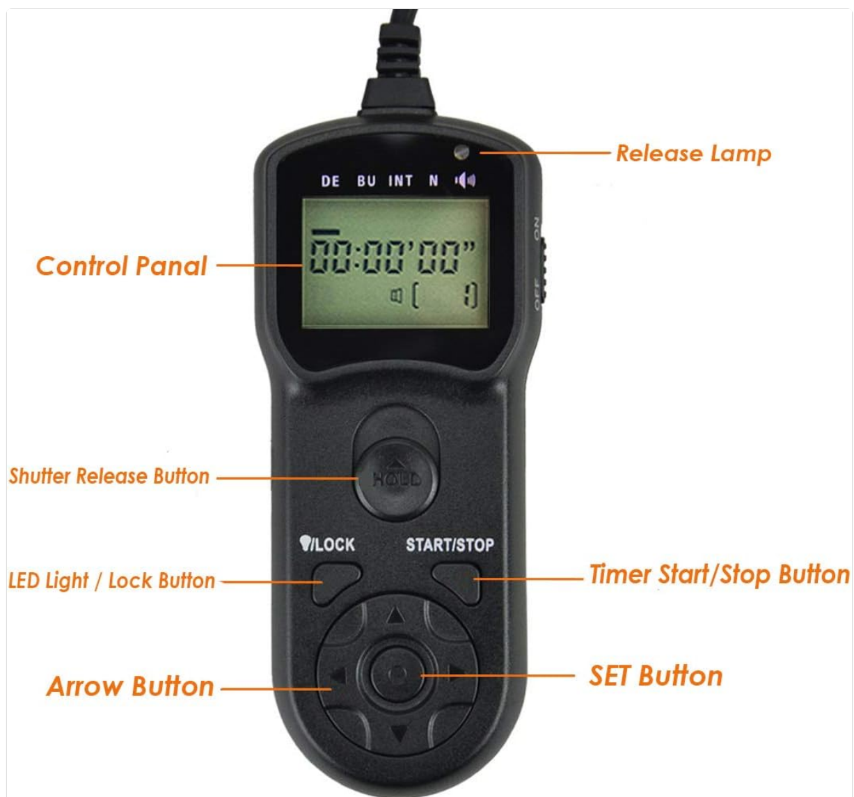
Figure 2: Labeled control panel of the JJC TM-M remote, highlighting the Shutter Release Button, LED Light/Lock Button, Arrow Buttons, Timer Start/Stop Button, and SET Button.
