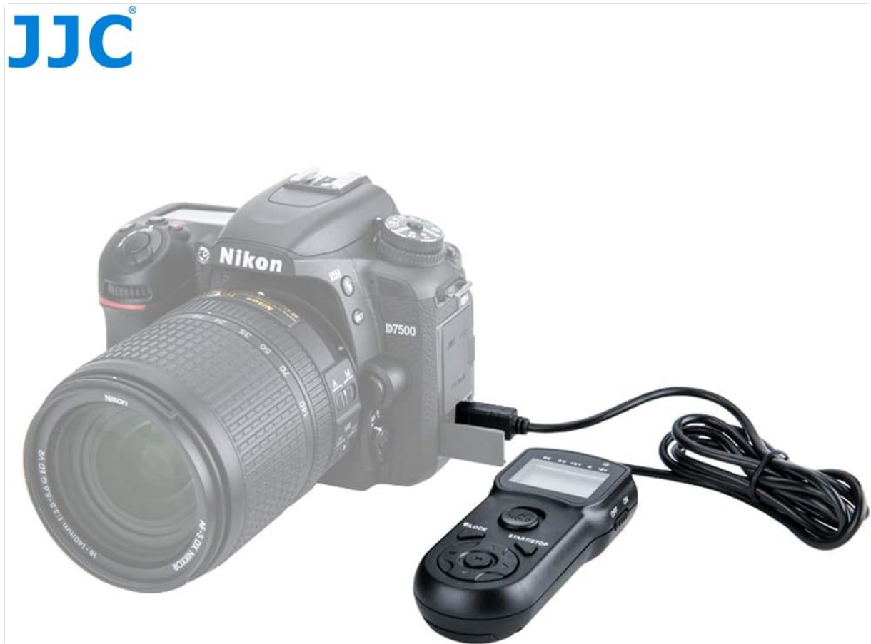
Figure 4: The JJC TM-M remote connected to a Nikon D7500 camera, ready for use.
