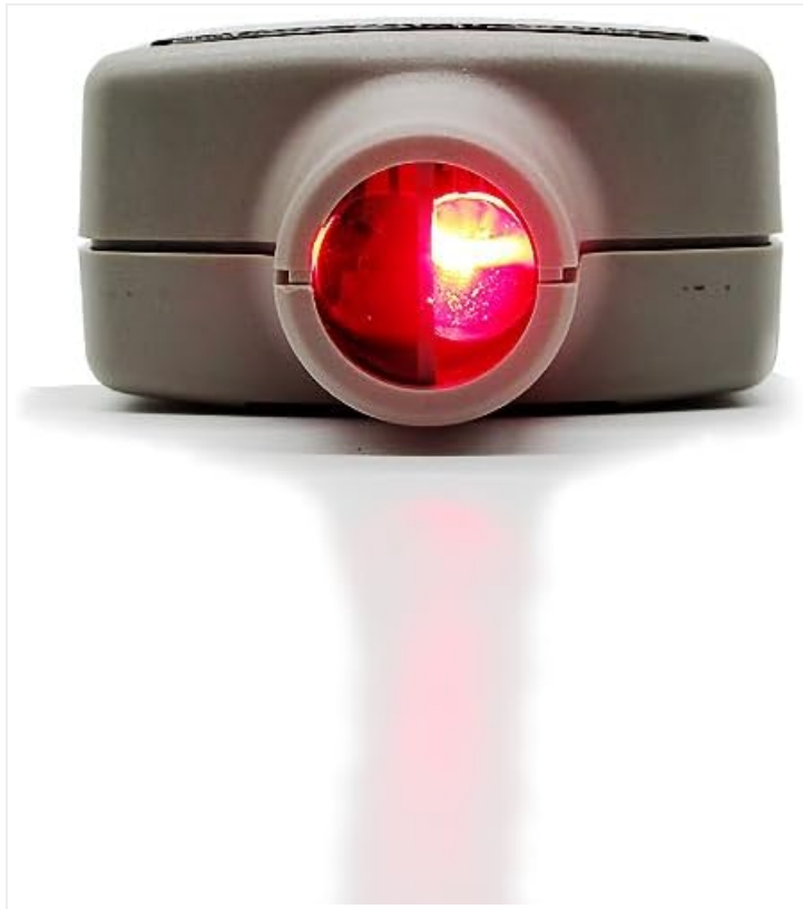
Figure 3.3: Front view showing the laser beam emitted from the sensor for targeting the reflective tape.
