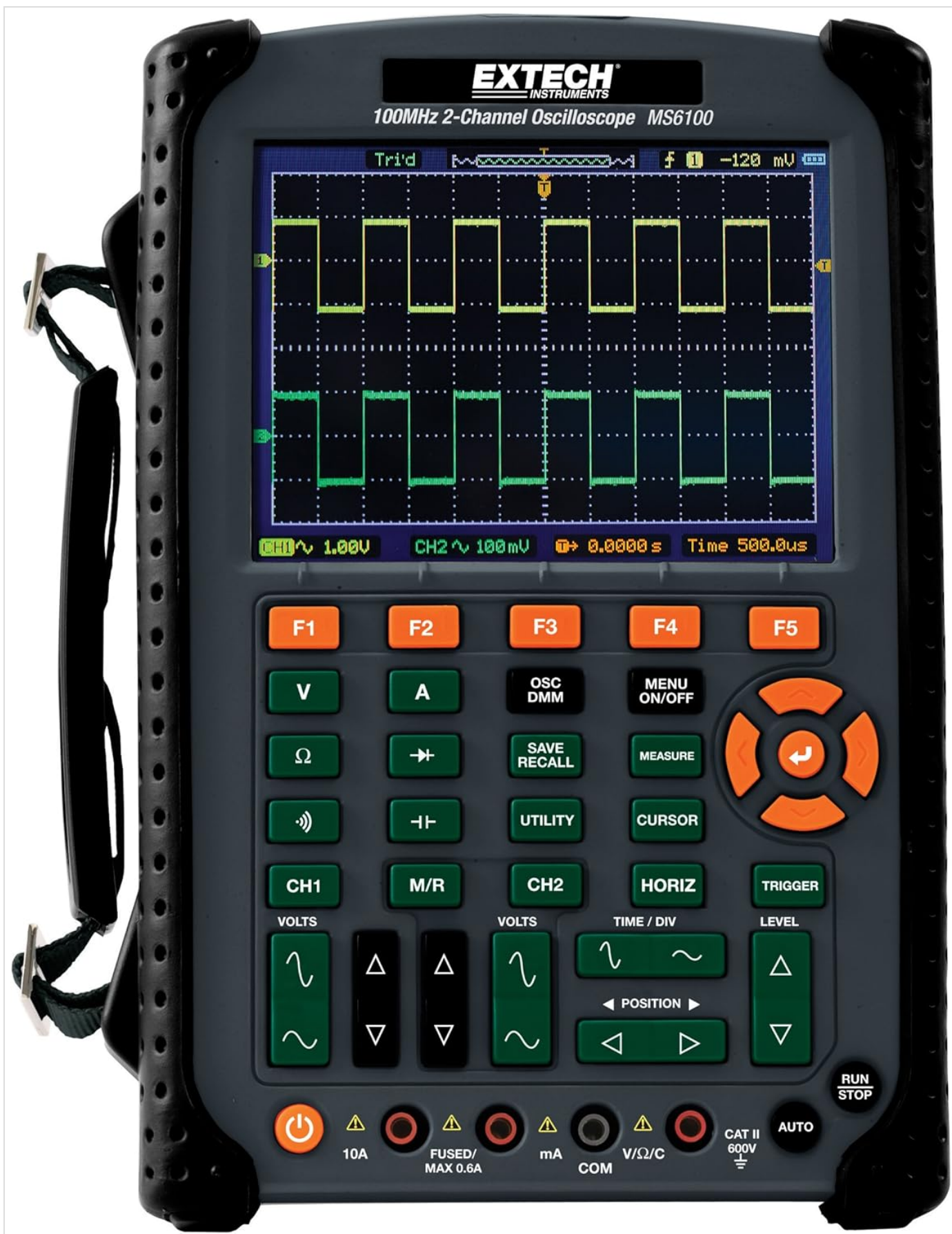
Figure 3.1: Front view of the Extech MS6100 Digital Oscilloscope, showing the color LCD display, function buttons (F1-F5), navigation controls, input terminals (10A, FUSED/MAX 0.6A, mA, COM, V/Ω/C, CAT II 600V), and dedicated buttons for oscilloscope and multimeter functions.
