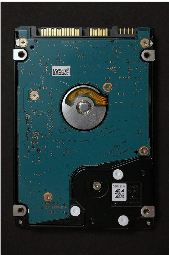
Figure 2: Back view of the Toshiba MQ01ABD050 hard drive, revealing the green circuit board (PCB) and the central motor assembly. Various electronic components, solder points, and screw mounts are visible. A QR code and a serial number (G3E12214) are also present on the PCB.
