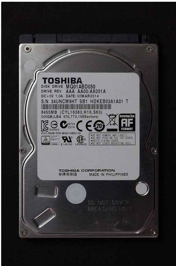
Figure 1: Front view of the Toshiba MQ01ABD050 hard drive. The label displays key information including the model number (MQ01ABD050), drive revision, power requirements (DC+5V 1.0A), manufacturing date (30MAR2014), and serial number (34UNCM9HTSB1). It also indicates the capacity (500GB) and various certifications. A warning advises not to remove the label or cover the breathing hole.
