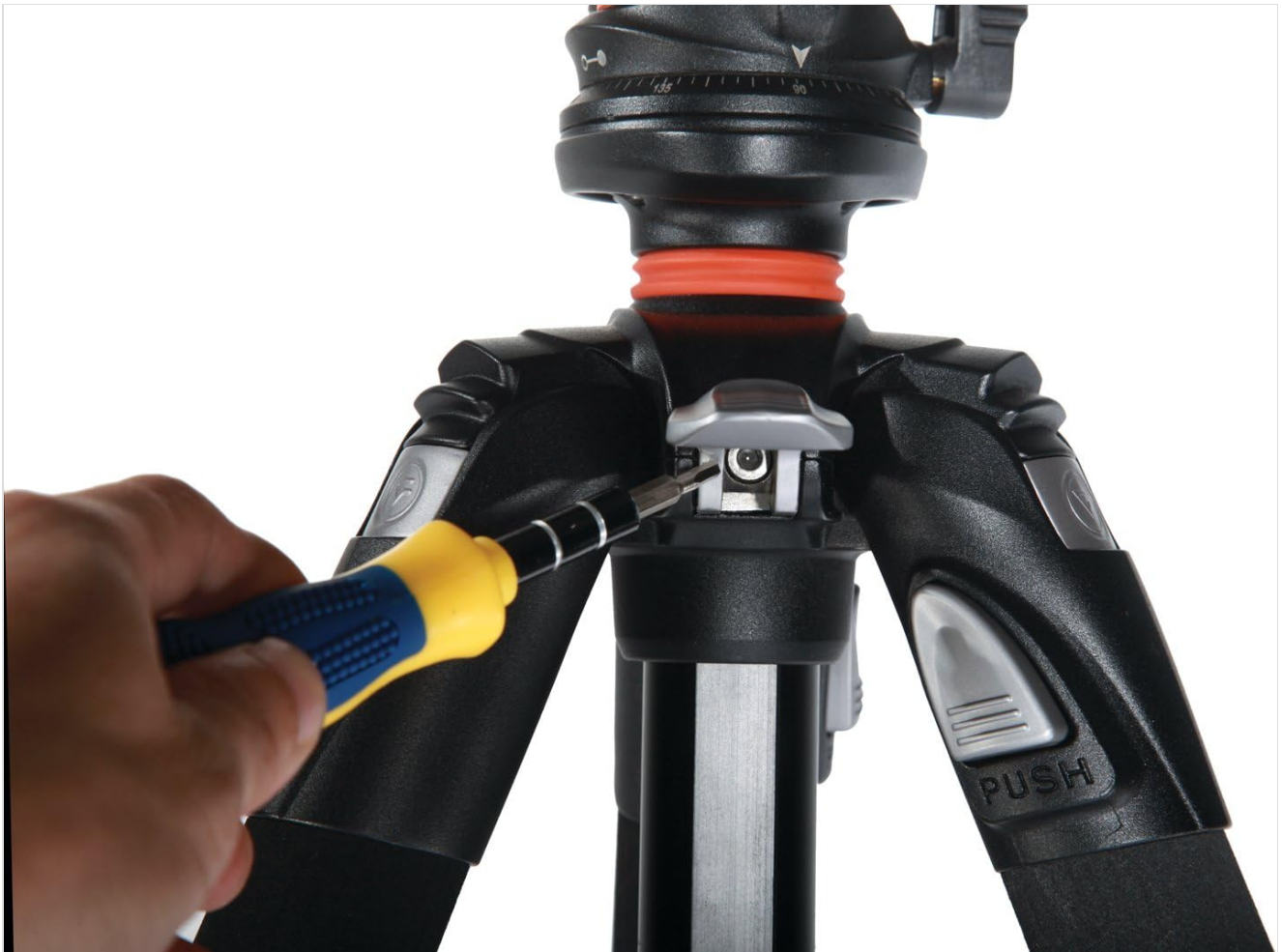
Image: A hand using a screwdriver to adjust the tension of a leg lock on the VANGUARD Abeo Plus 323CB tripod.
