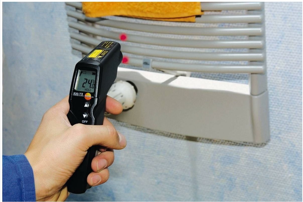
Figure 3: The Testo 830-T1 in use, measuring the surface temperature of a radiator.
