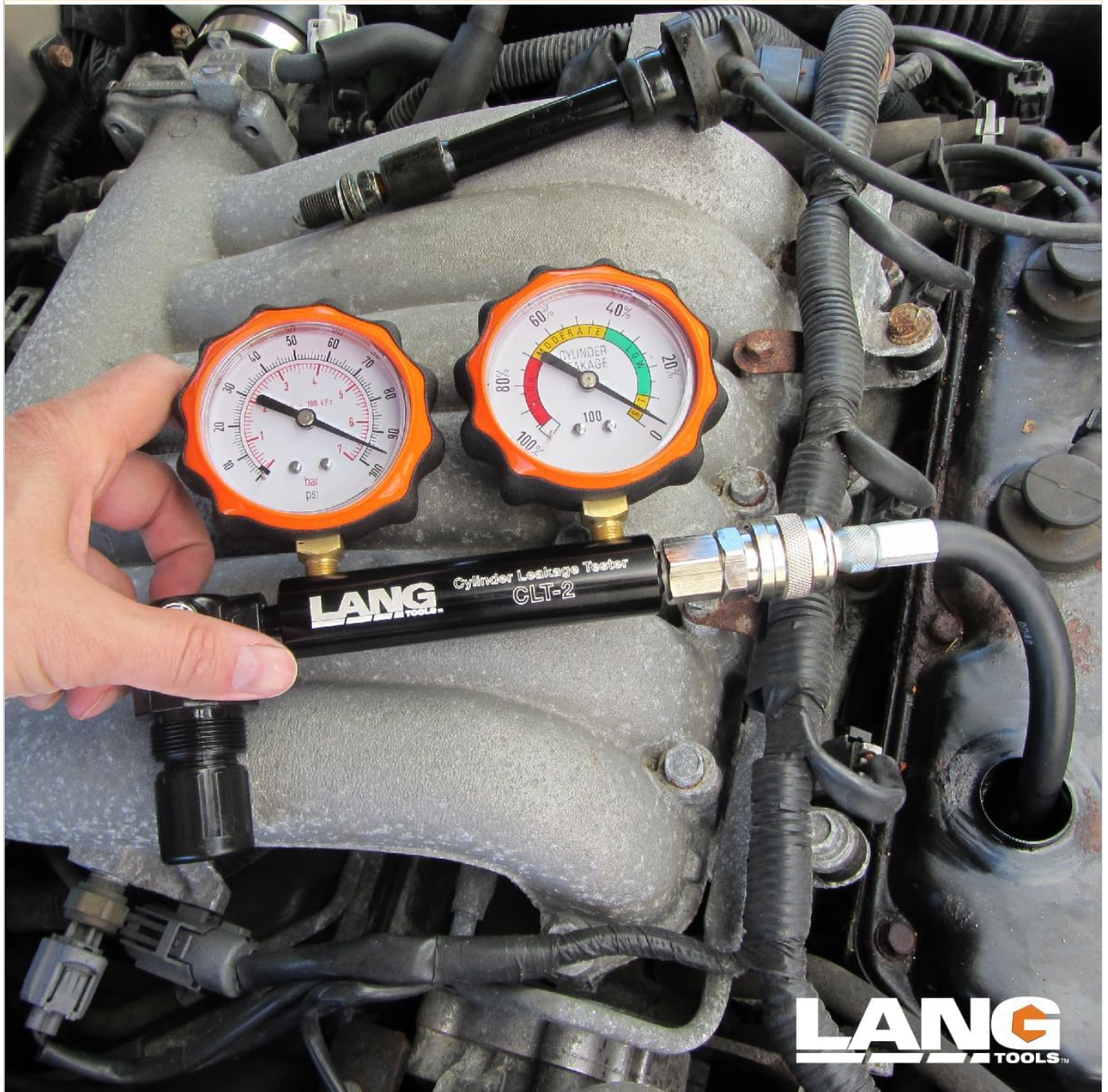
Figure 6.1: The CLT-2 Cylinder Leakage Tester connected to an engine cylinder, demonstrating typical usage during a diagnostic procedure.
