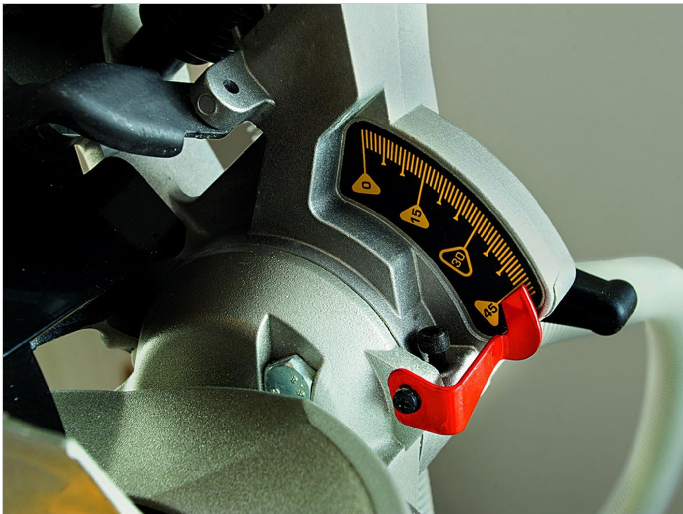
Figure 4.3.1: Bevel angle adjustment. Use the lever to set the saw head to the required bevel angle.
