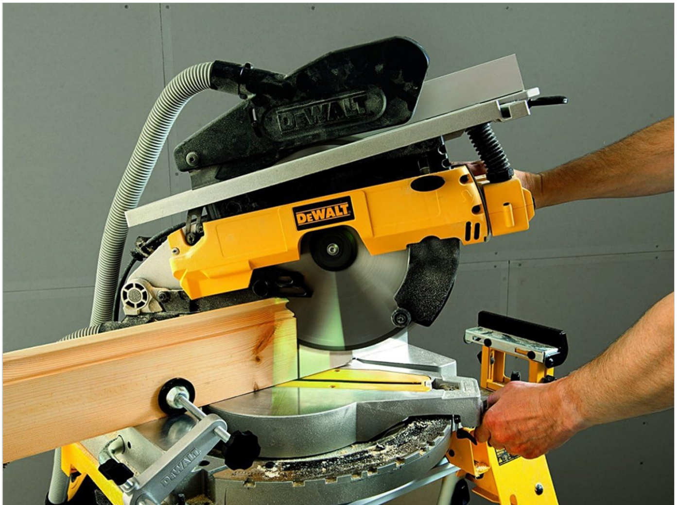
Figure 4.4.2: Performing a miter cut. The saw's design allows for precise angled cuts.
