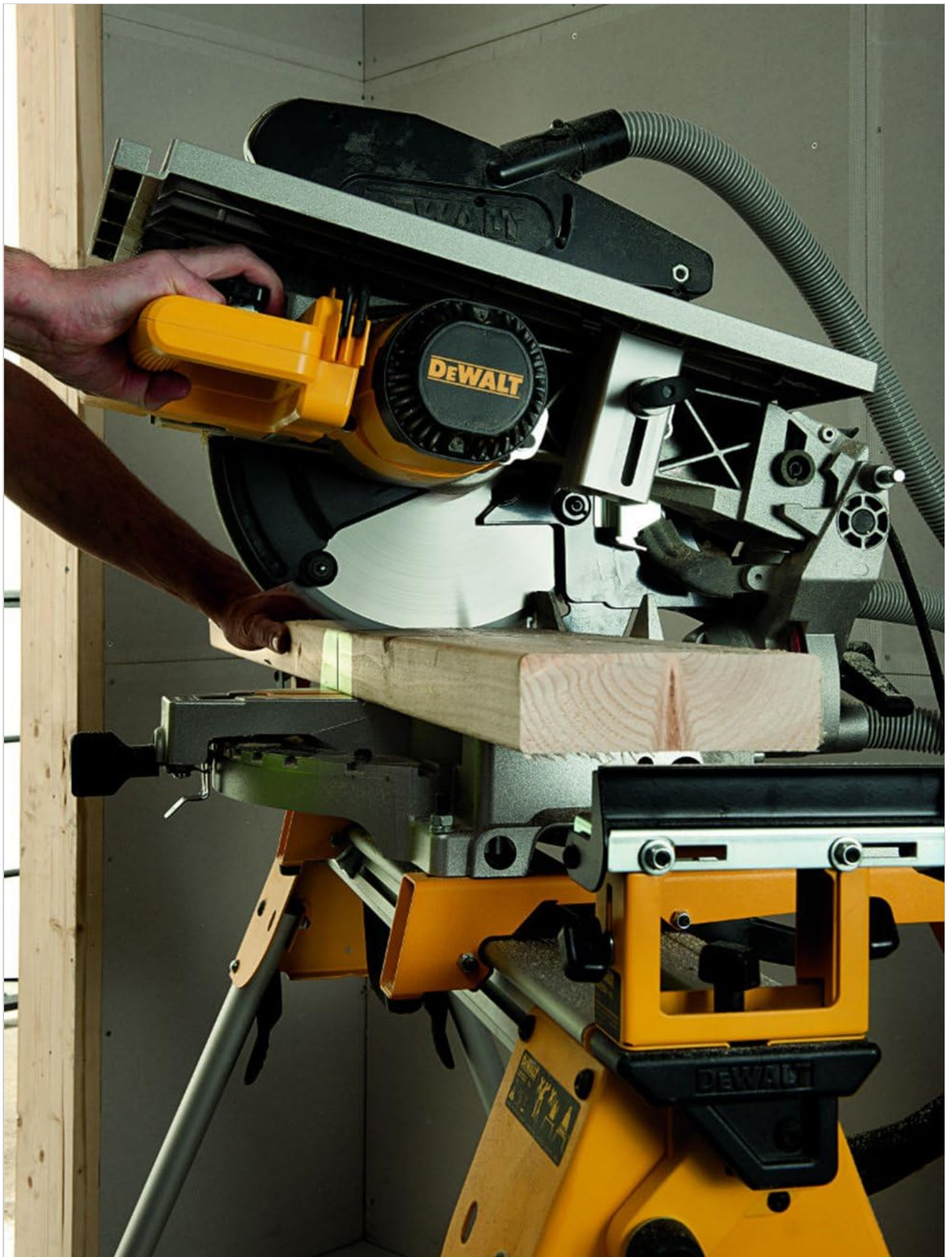
Figure 4.4.1: Performing a cross-cut. Ensure the workpiece is stable and the blade is aligned with the cut line.
