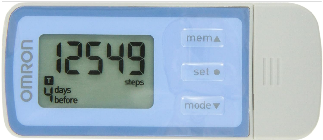
Image: The Omron Tri-Axis Pedometer's digital display showing a step count of 12,549, along with "4 days before" indicating memory recall. Buttons for "mem", "set", and "mode" are visible.
