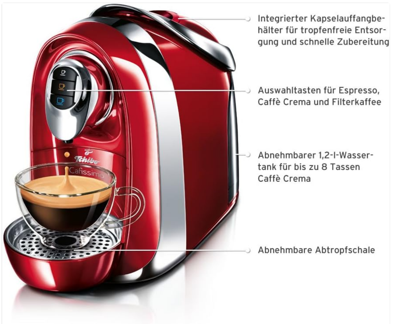
Image 3.1: Overview of the Tchibo Cafissimo Compact machine with key components labeled. This includes the integrated capsule collector, selection buttons for Espresso, Caffè Crema, and Filter Coffee, the removable 1.2-liter water tank, and the removable drip tray.
