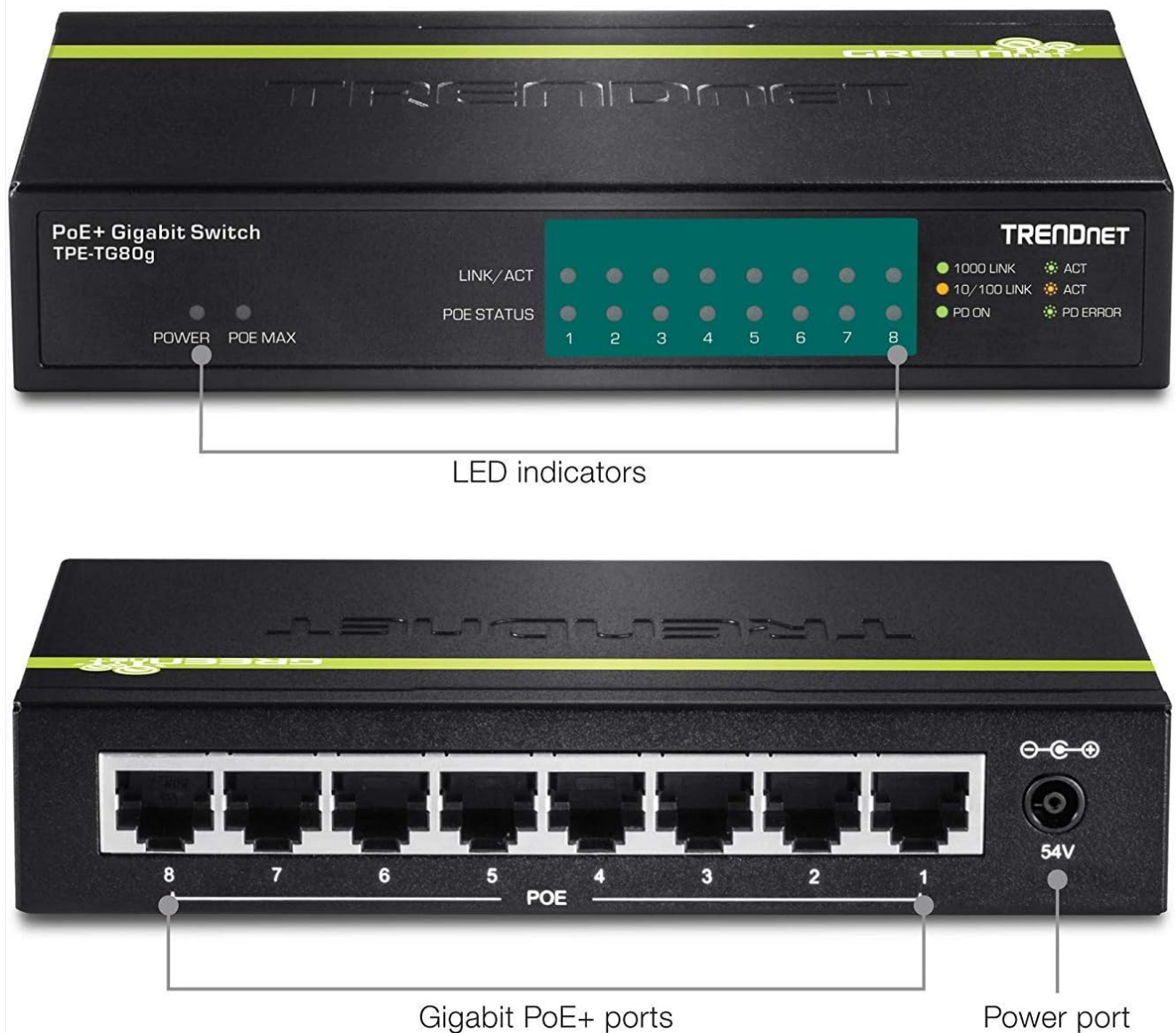
Figure 2: Front and Back Panels with LED Indicators and Ports
