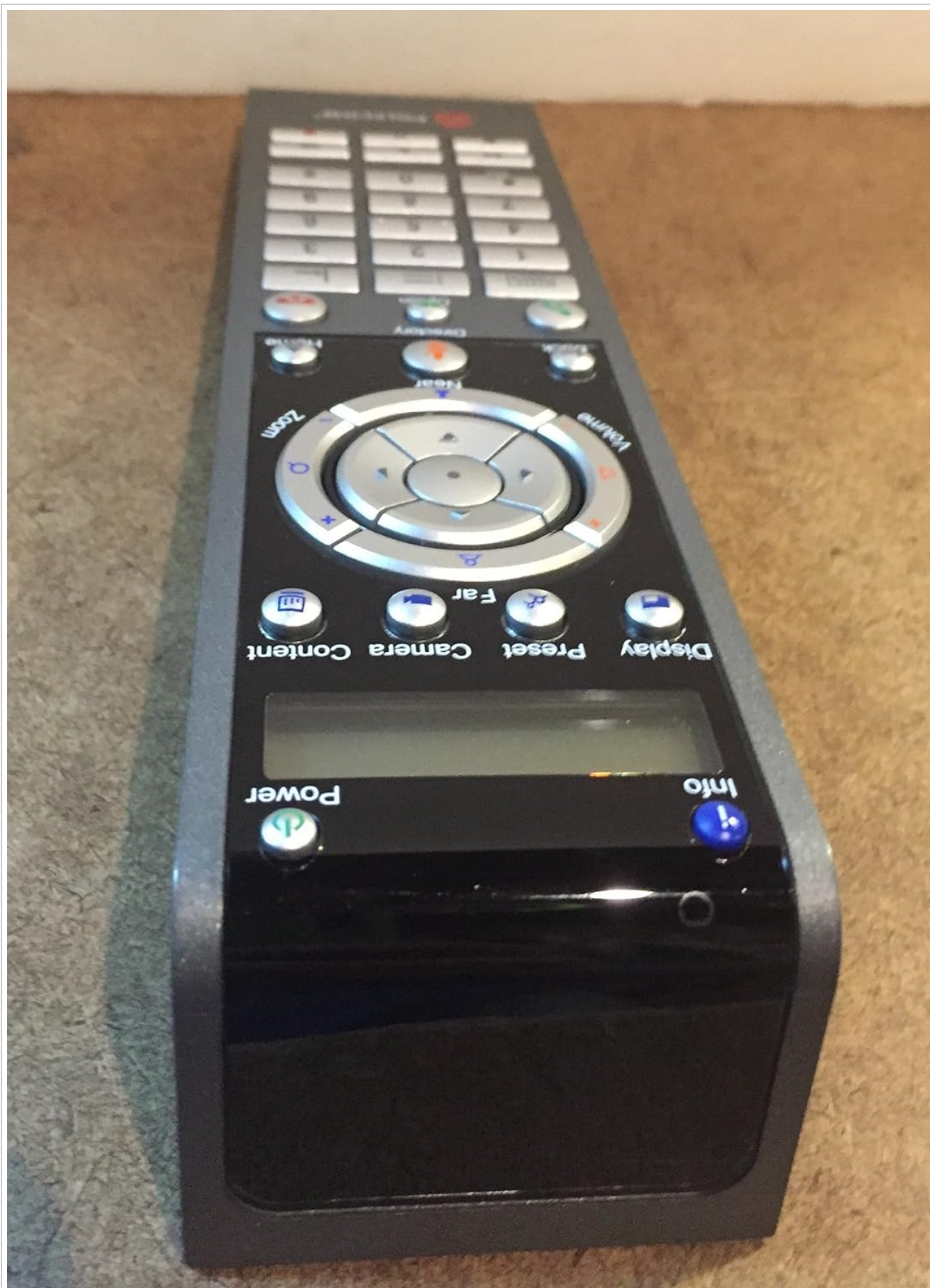
Figure 3: The Polycom HDX 7000 system remote control, used for navigating menus, controlling calls, and adjusting camera settings.
