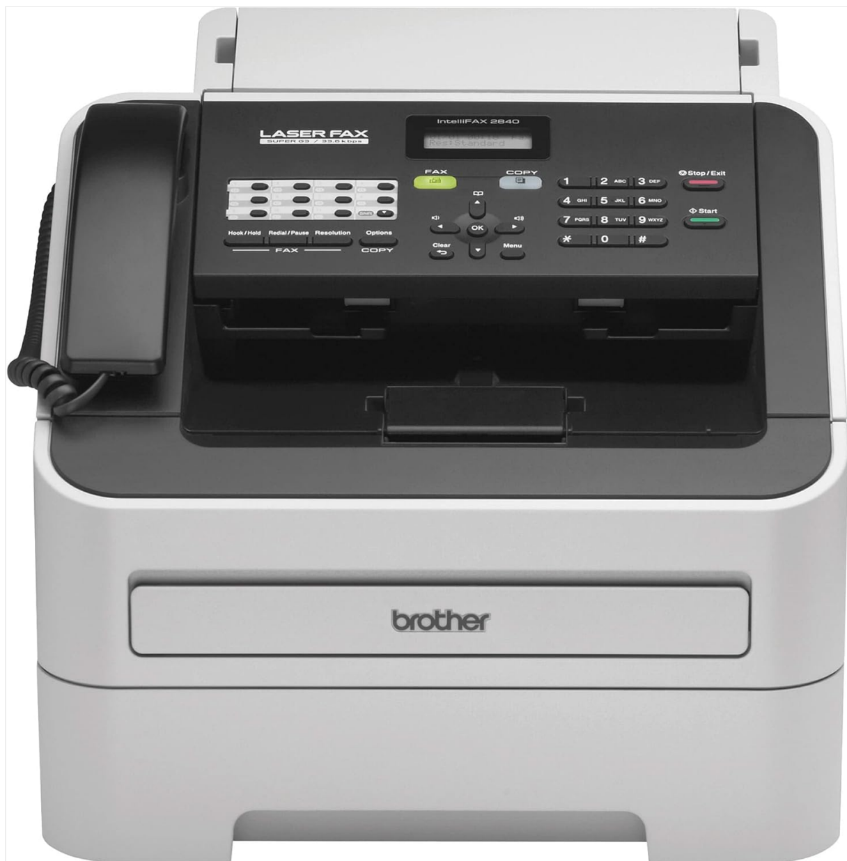
Figure 3.1: The control panel features a display, numeric keypad, function buttons, and navigation keys.
