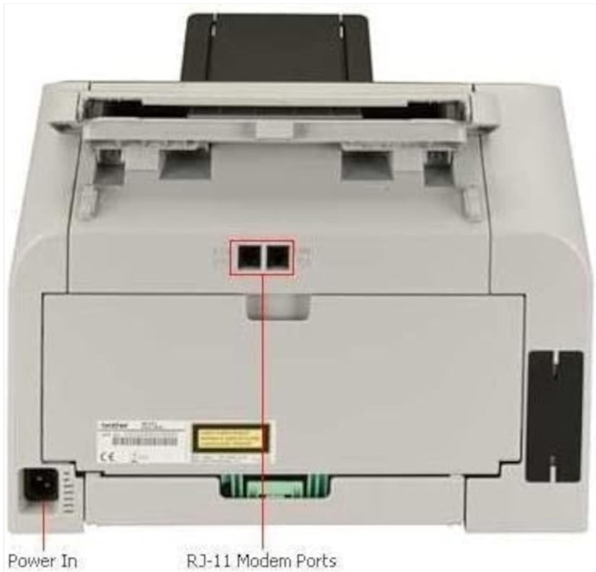
Figure 2.1: Rear view illustrating power input and RJ-11 modem ports for telephone line connections.
