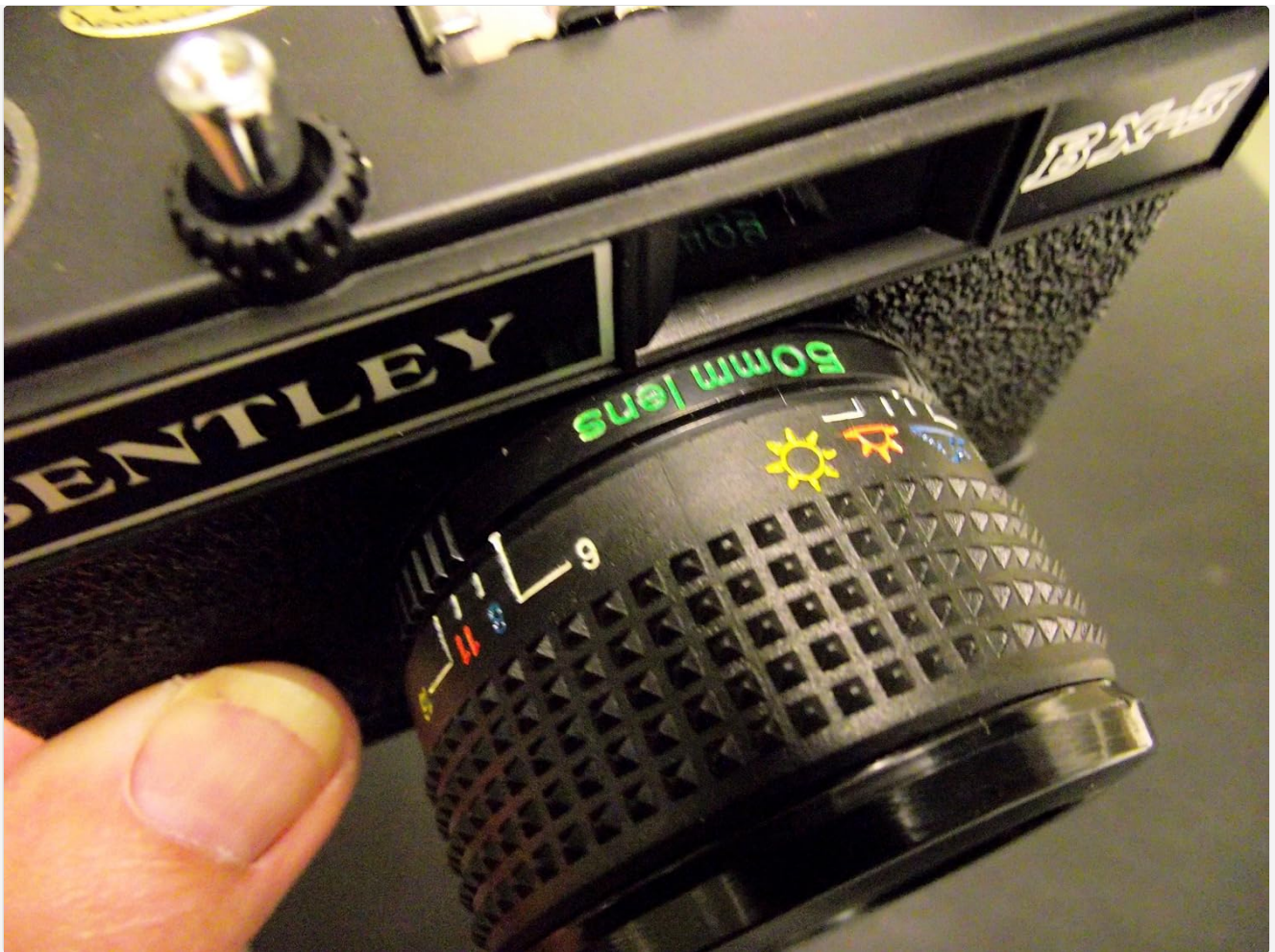
Figure 3.1: Detail of the 50mm lens, showing the focus ring and aperture settings, which may include symbols for different lighting conditions.
