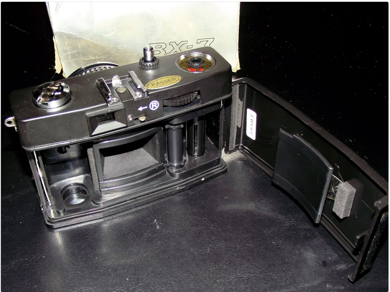
Figure 2.1: The camera back opened, revealing the film loading compartment, take-up spool, and film canister chamber.
