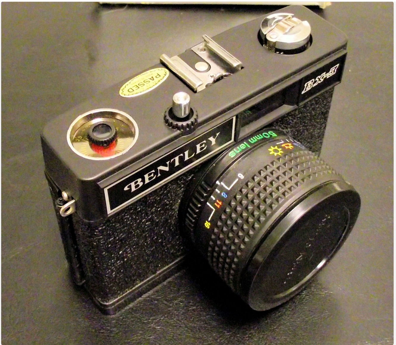
Figure 1.1: The Bentley BX-3 35mm Camera with its 50mm optical glass lens attached. This image shows the camera's front view, highlighting the lens, viewfinder, and film advance knob.
