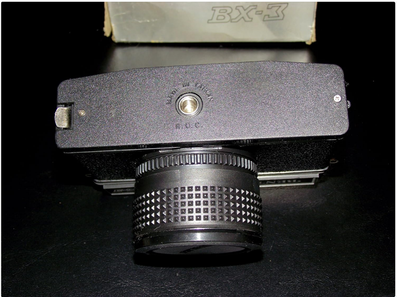
Figure 6.1: The bottom of the Bentley BX-3 camera, showing the tripod mount and film rewind release.
