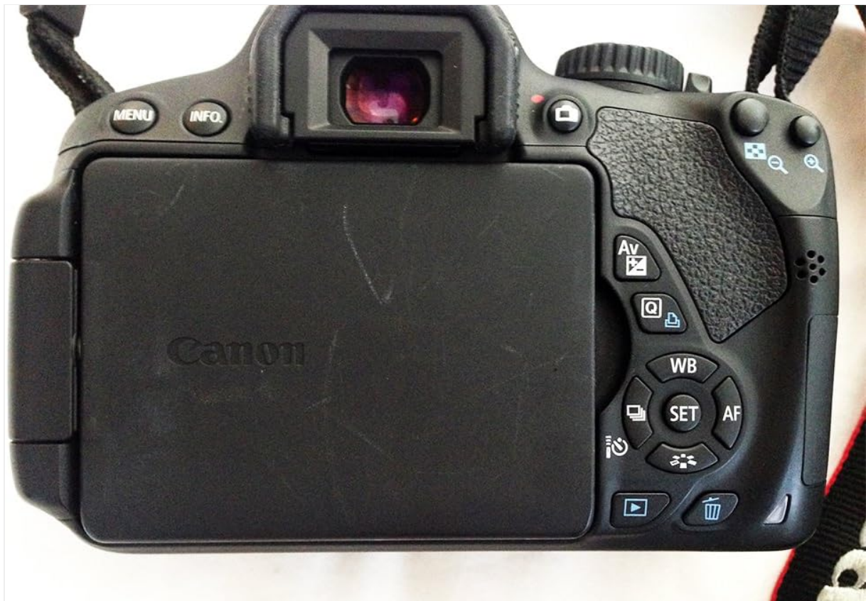
Image: Rear view of the Canon EOS 650D, showing the touchscreen LCD and control buttons.
