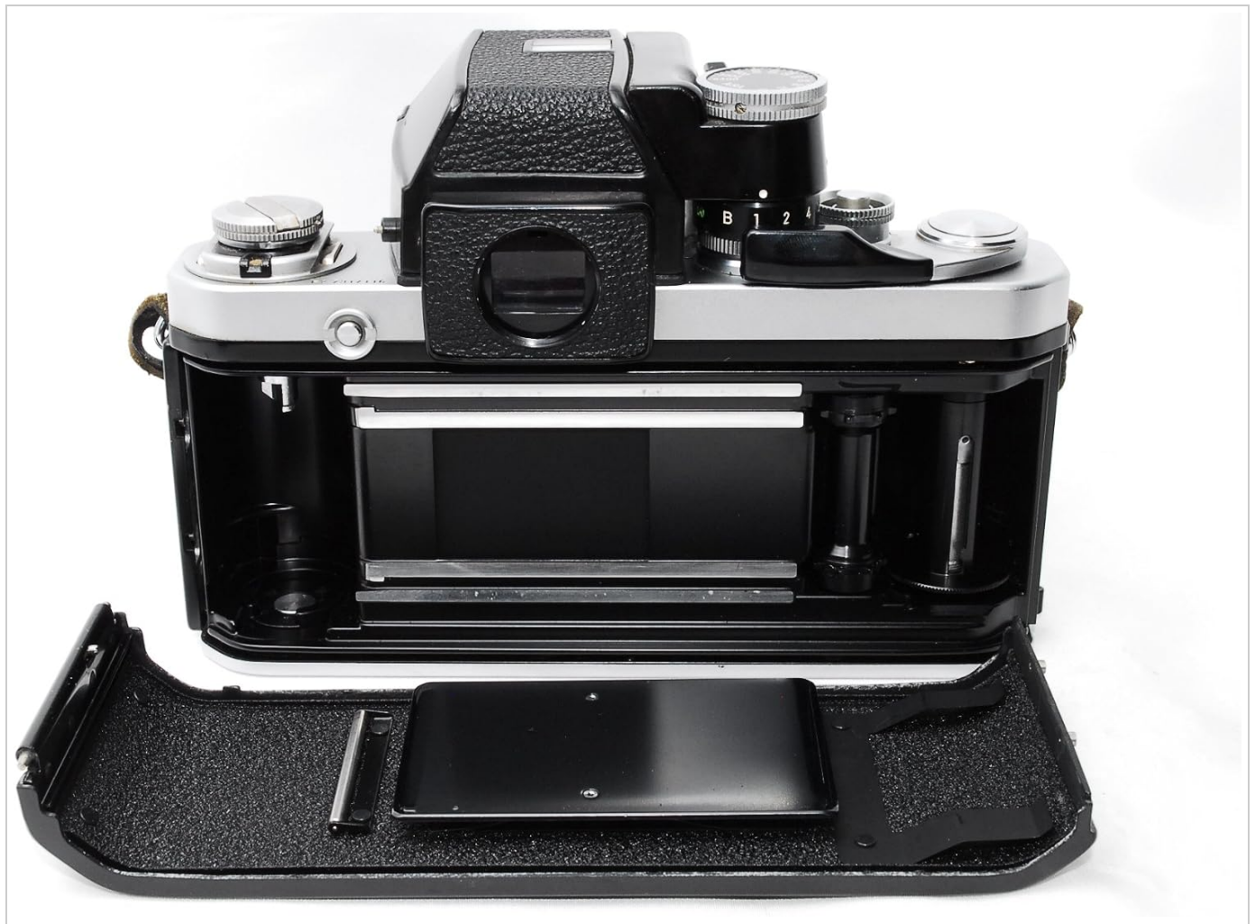
Image: The Nikon F2 Photomic camera with its back open, revealing the film chamber on the left and the take-up spool on the right, ready for film loading.
