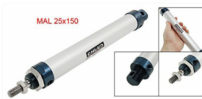
Figure 2: Detailed views of the uxcell MAL 25x150 Pneumatic Cylinder. This composite image shows the overall cylinder, a close-up of the air inlet port, and the threaded piston rod with its securing nut, illustrating key connection points and the compact size when held in hand.
