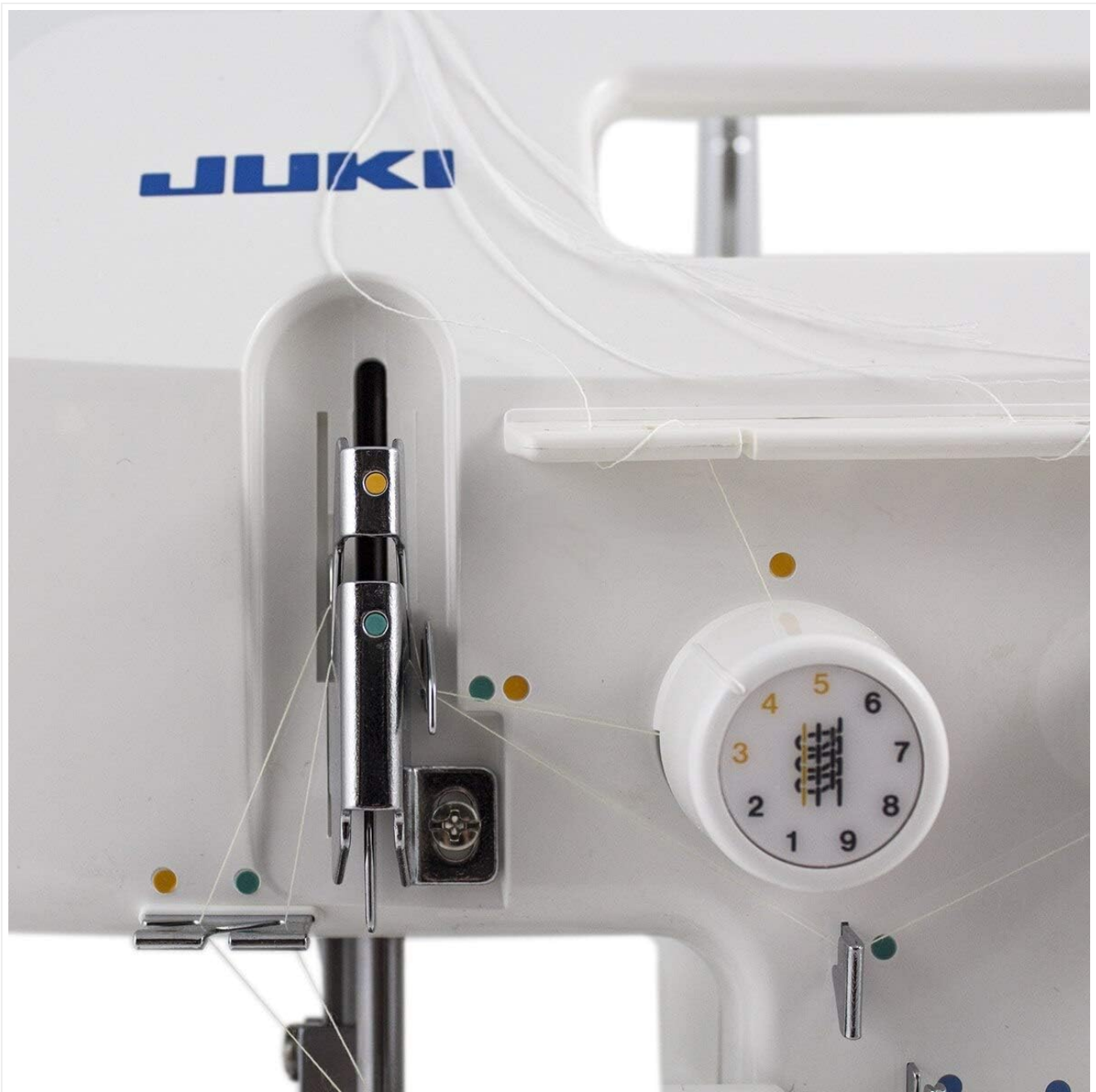
Figure 3.2: Needle and Looper Threading Area. This image shows a close-up of the needle bar and looper threading guides, highlighting the intricate path threads must follow.
