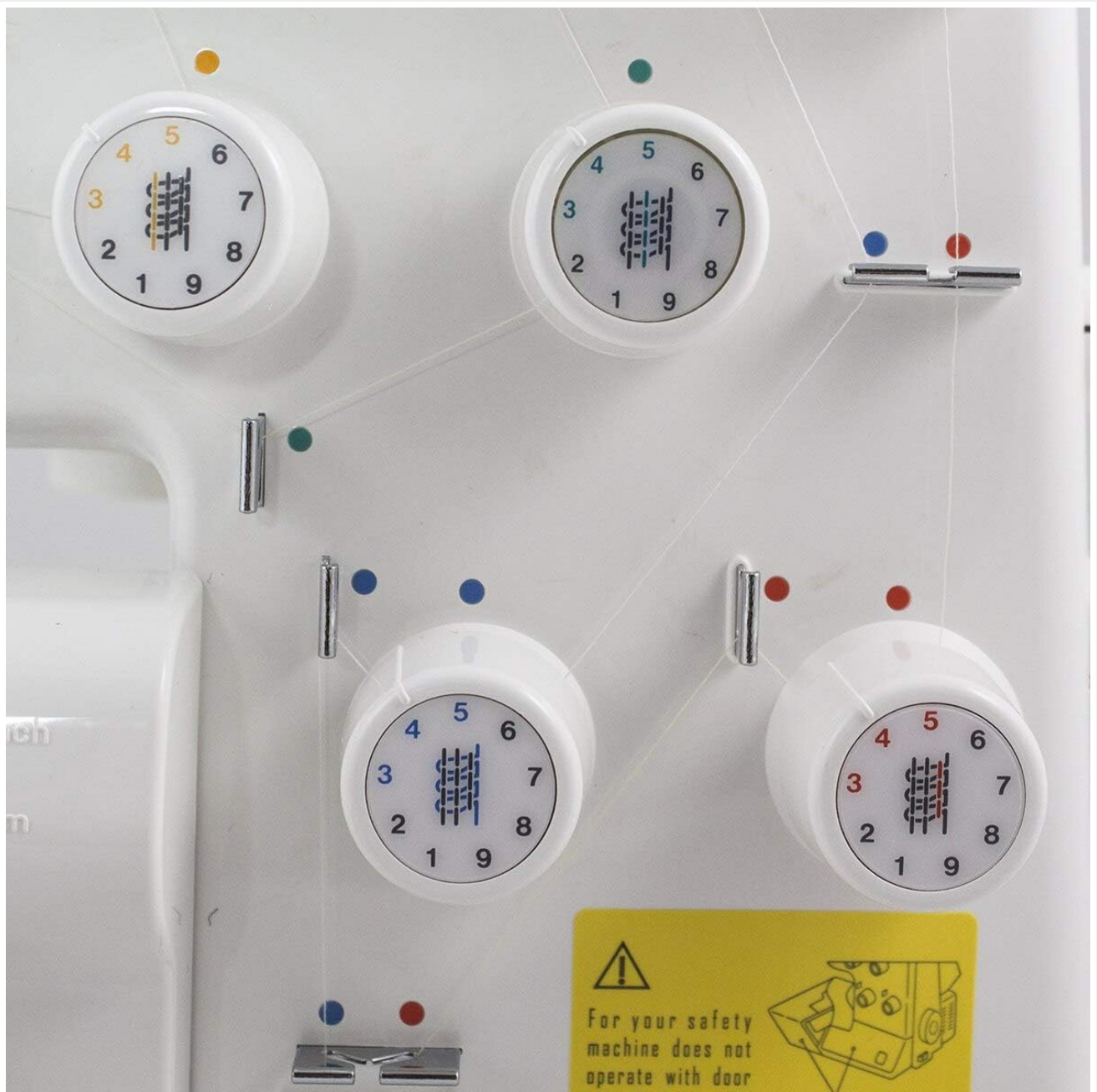
Figure 3.1: Thread Tension Dials. This image displays the four color-coded tension dials on the Juki MO-654DE, essential for proper stitch formation.
