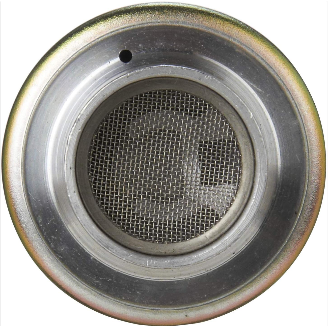
Image 3.4: Bottom view of the fuel pump, showing the fuel inlet and integrated strainer.
