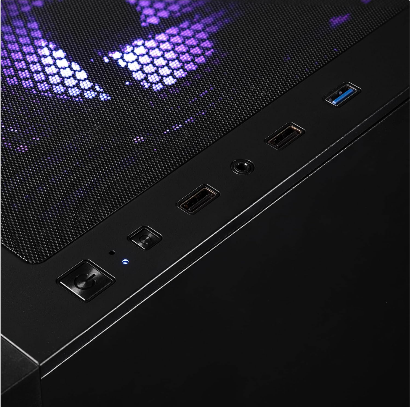
Figure 2.1: Top panel connectivity ports, including USB 3.0, USB 2.0, and audio jacks.
