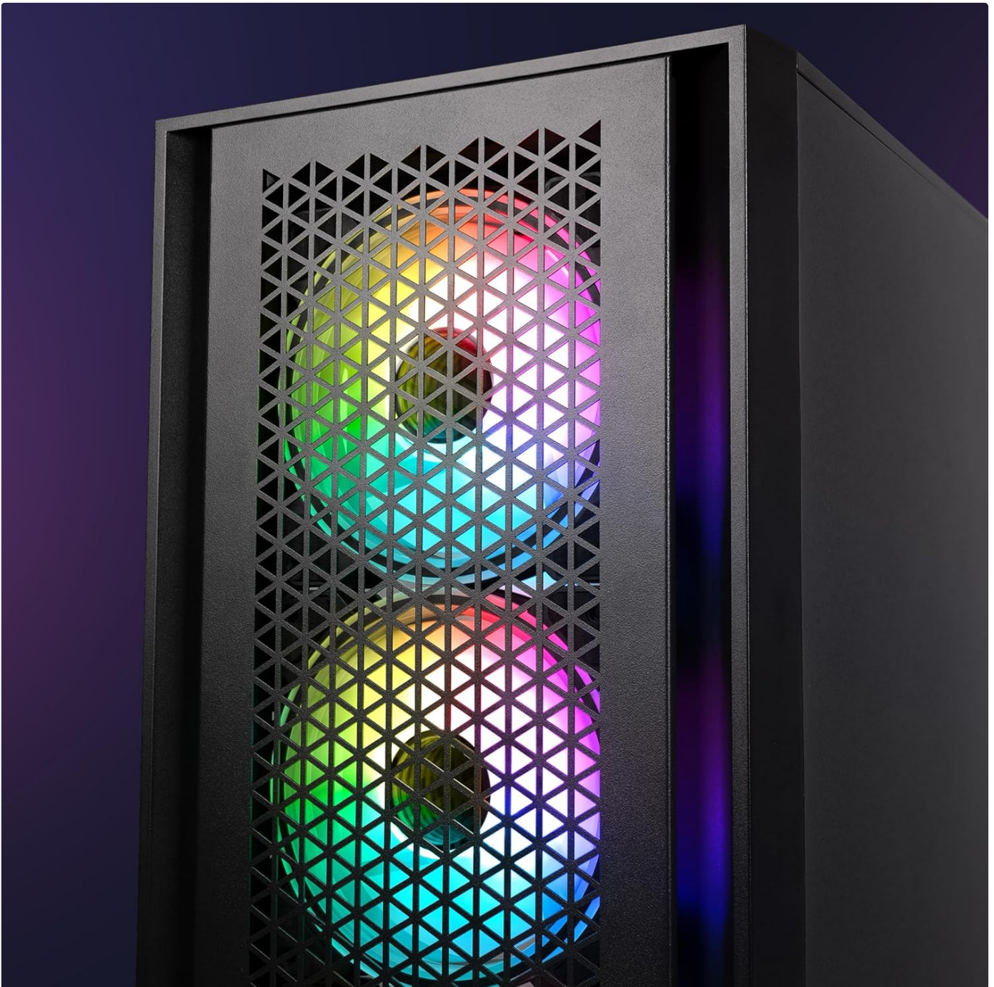
Figure 4.1: Front panel fans, crucial for system cooling. Regular cleaning of these vents is recommended.
