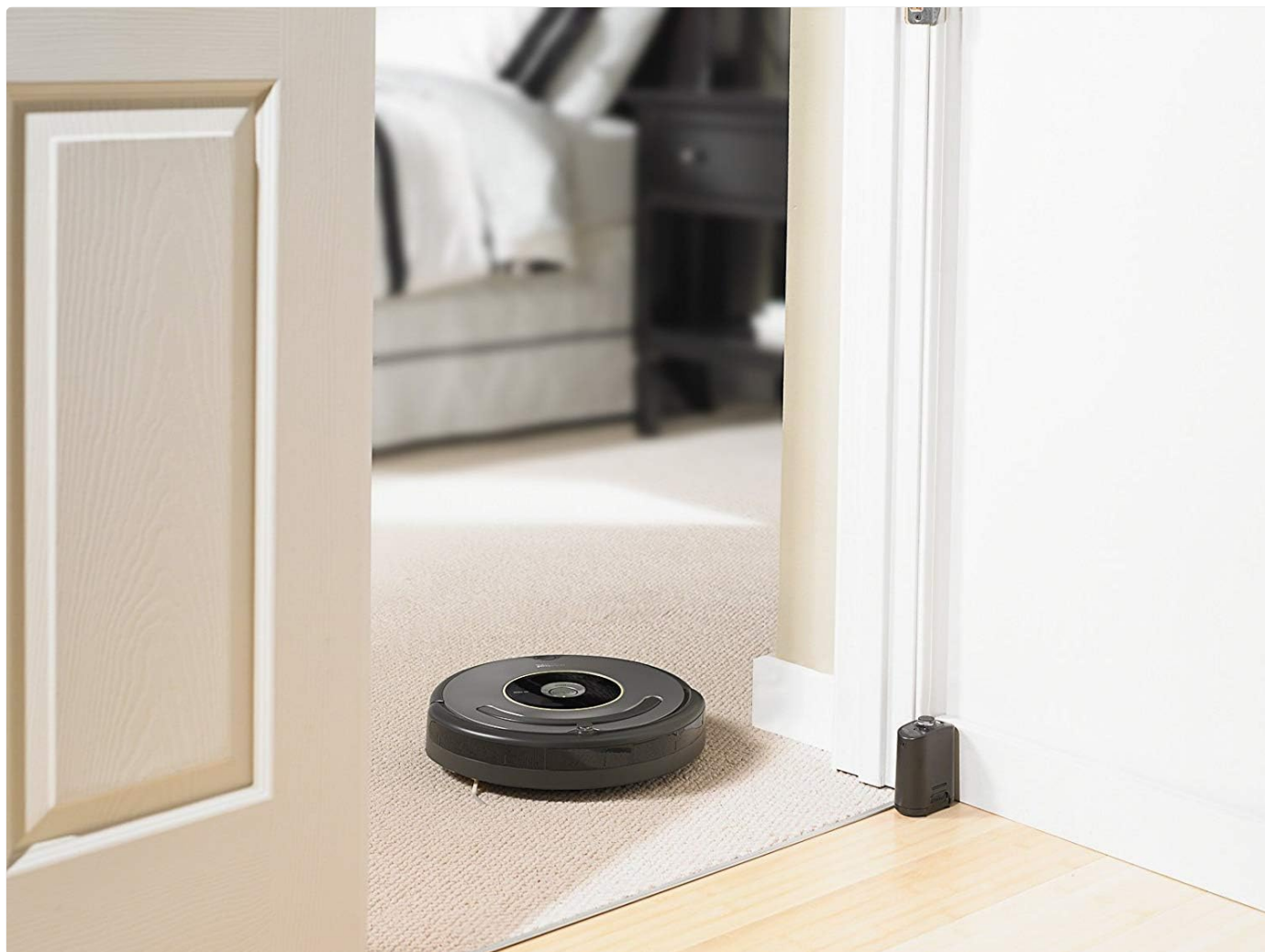
Figure 4: A Virtual Wall creates an invisible barrier to guide Roomba's cleaning path.
