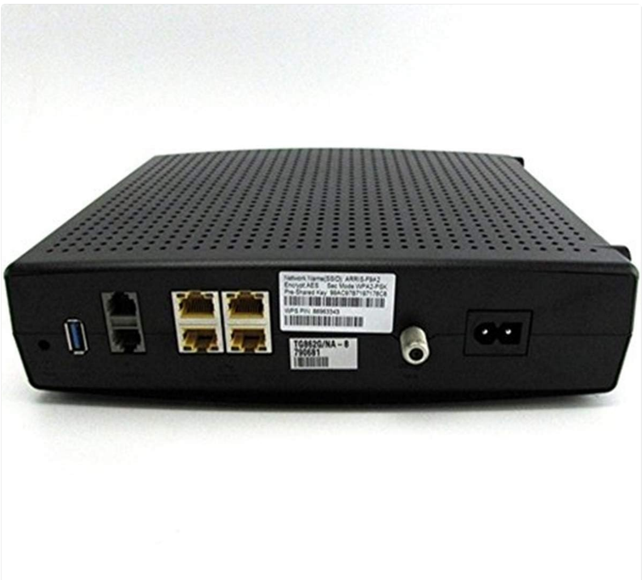
Figure 3.2.1: Rear view of the ARRIS TG862G showing connection ports. From left to right: USB port, four Ethernet ports, two
