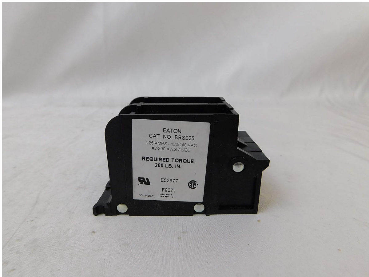
Image: A side view of the Eaton BRS225 lug kit, highlighting the product label. The label specifies "EATON CAT. NO. BRS225", "225 AMPS - 120/240 VAC", "#2-300 AWG AL/CU", and "REQUIRED TORQUE: 200 LB. IN."
