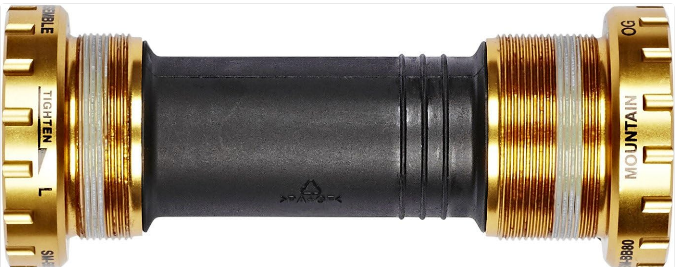
Figure 4: A compatible SHIMANO SM-BB80 bottom bracket, typically used with the FC-M820 crankset. Note the gold-colored cups and central sleeve.
