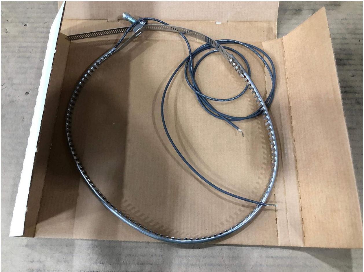
Figure 3.1: The MARS TUTCO CH-101 Compressor Heater as received in its cardboard packaging. The heater consists of a flexible metal band with an integrated heating element and electrical leads, secured by a hose clamp mechanism.
