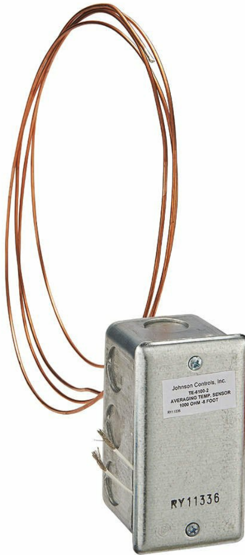
Figure 1: Johnson Controls TE-6100-2 Nickel Temperature Sensing Element. This image shows the metallic conduit box with an attached label indicating "TE-6100-2 AVERAGING TEMP. SENSOR 1000 OHM-8 FOOT" and several copper wires extending from the top, coiled for an 8-foot averaging length.
