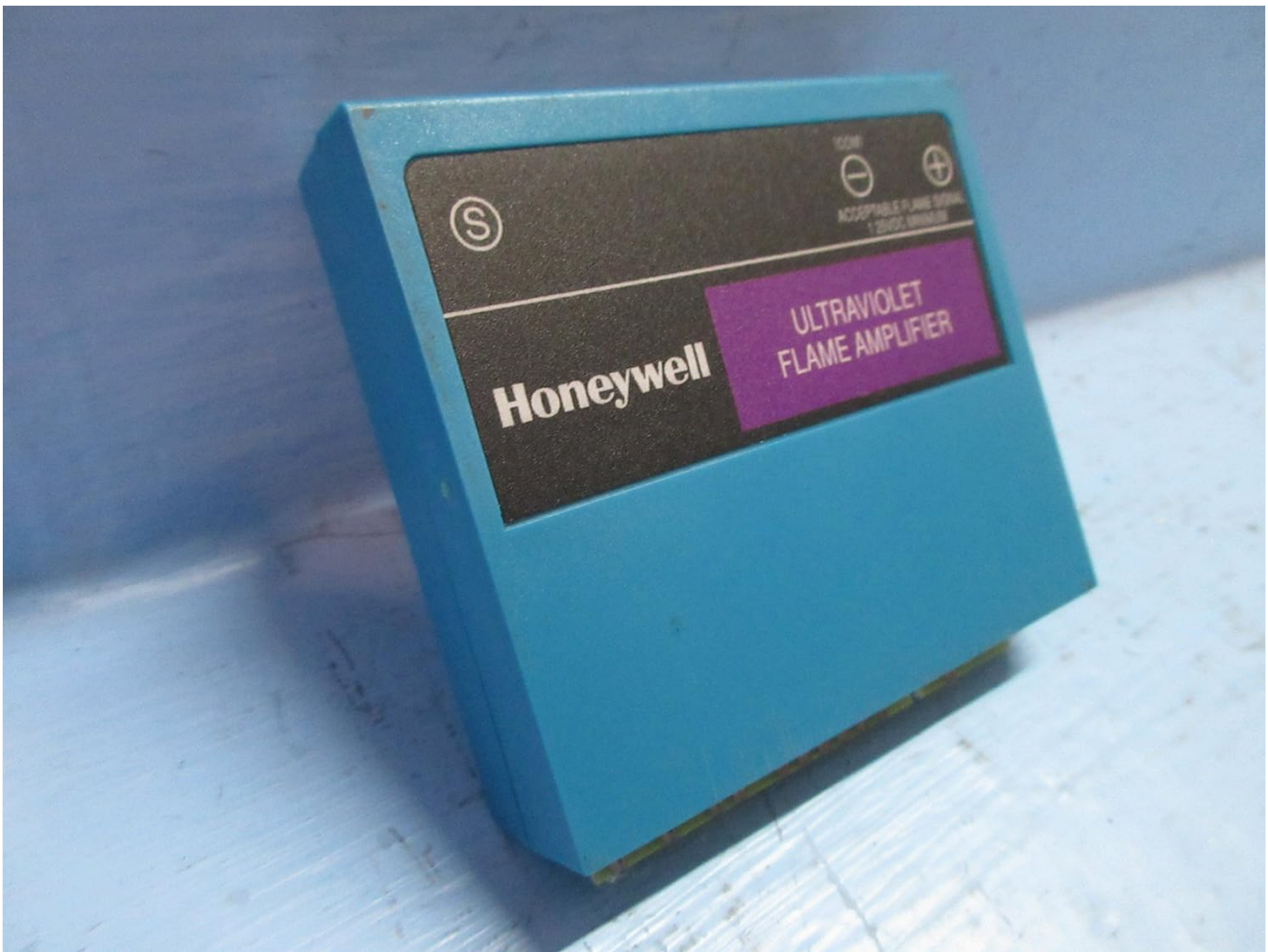
Figure 1: Angled view of the Honeywell Ultraviolet Flame Amplifier (R7849A1015). The device is blue with a black and purple label indicating "Honeywell" and "ULTRAVIOLET FLAME AMPLIFIER".
