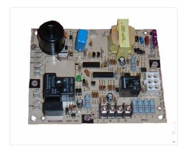
Image: The ADP 76722700 Control Board, showing various electronic components, relays, and connection terminals. This board is essential for regulating the functions of a unit heater.
