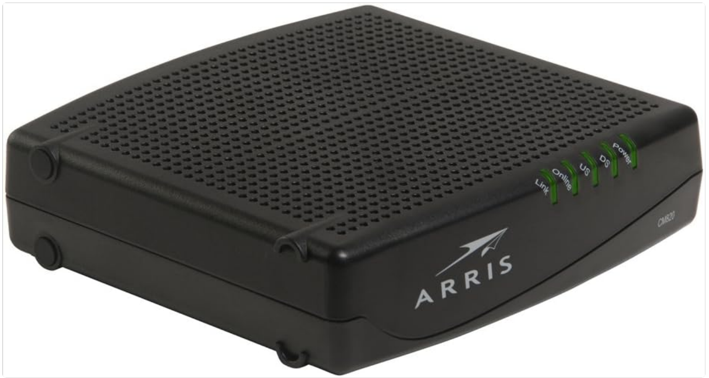
Figure 1: Front view of the ARRIS CM820A Cable Modem. Visible indicators include Power, DS (Downstream), US (Upstream), Online, and Link.
