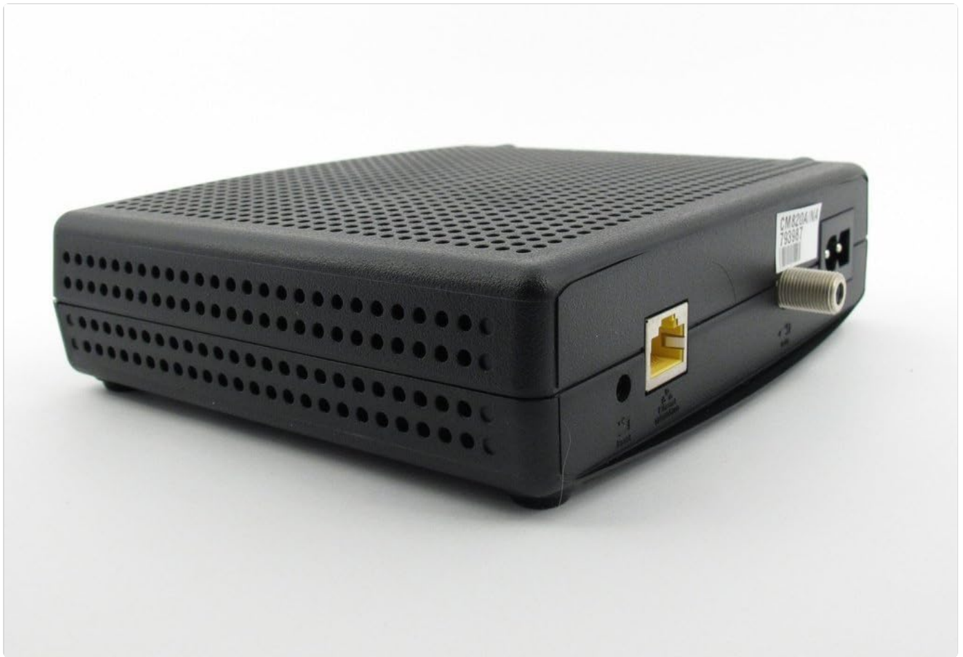
Figure 2: Rear view of the ARRIS CM820A Cable Modem. Ports include a coaxial cable connector, an Ethernet port, and a power input.
