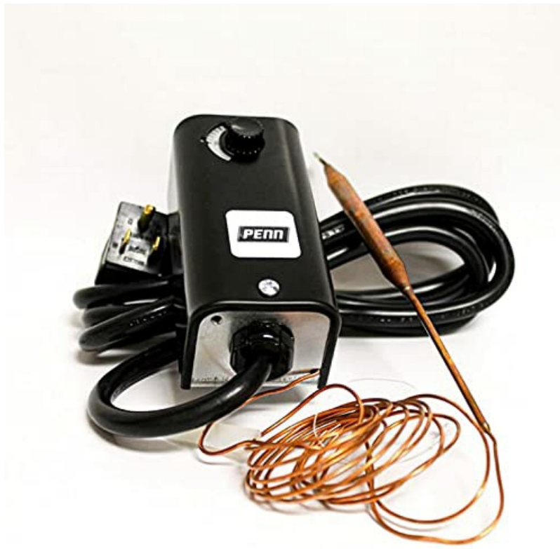
Image: The Johnson Controls A19AAT-2C Penn Series A19 Thermostat, showing its black housing, temperature adjustment dial, power cord with piggyback plug, and the coiled copper remote sensing bulb with its capillary tube.
