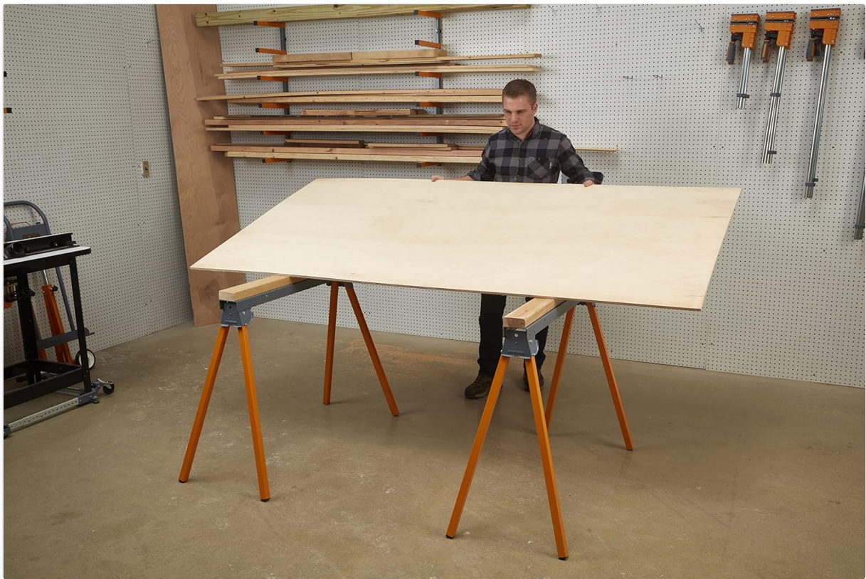
Figure 5: A large sheet of plywood is being placed across two unfolded sawhorses, demonstrating their utility as a stable platform for supporting wide workpieces. This setup is ideal for tasks requiring a broad and secure work area.
