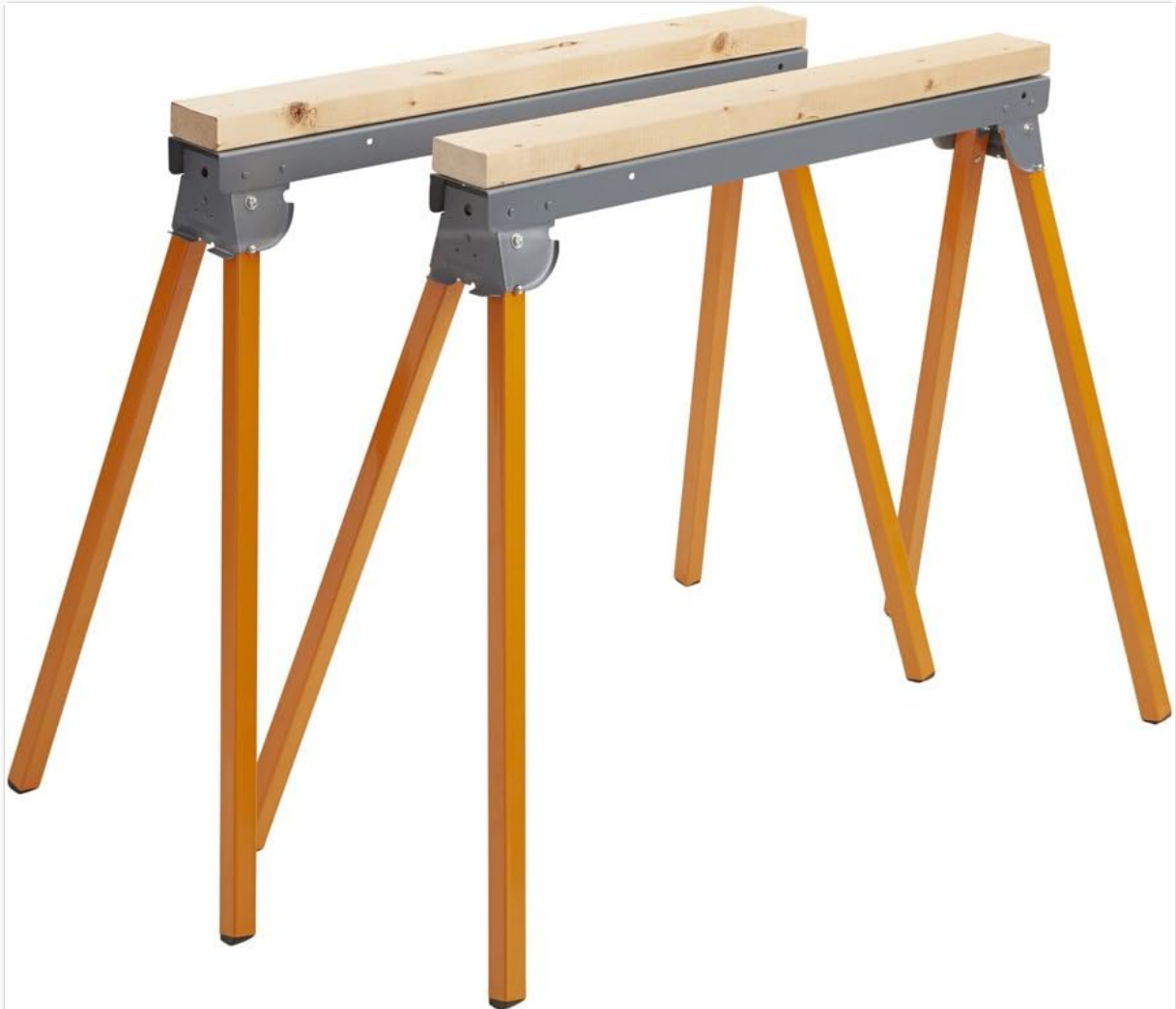
Figure 3: The sawhorses are shown with 2x4 wood pieces securely attached to their tops. This configuration provides a sacrificial surface for cutting and drilling, extending the life of the steel sawhorse tops.
