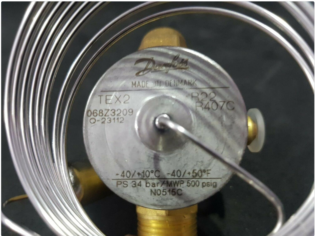
Figure 3.2: Close-up view of the valve's top plate, displaying model number (068Z3209), refrigerant type (R22/R407C), temperature range (-40/+10°C, -40/+50°F), and pressure ratings (PS 34 bar/MWP 500 psig).
