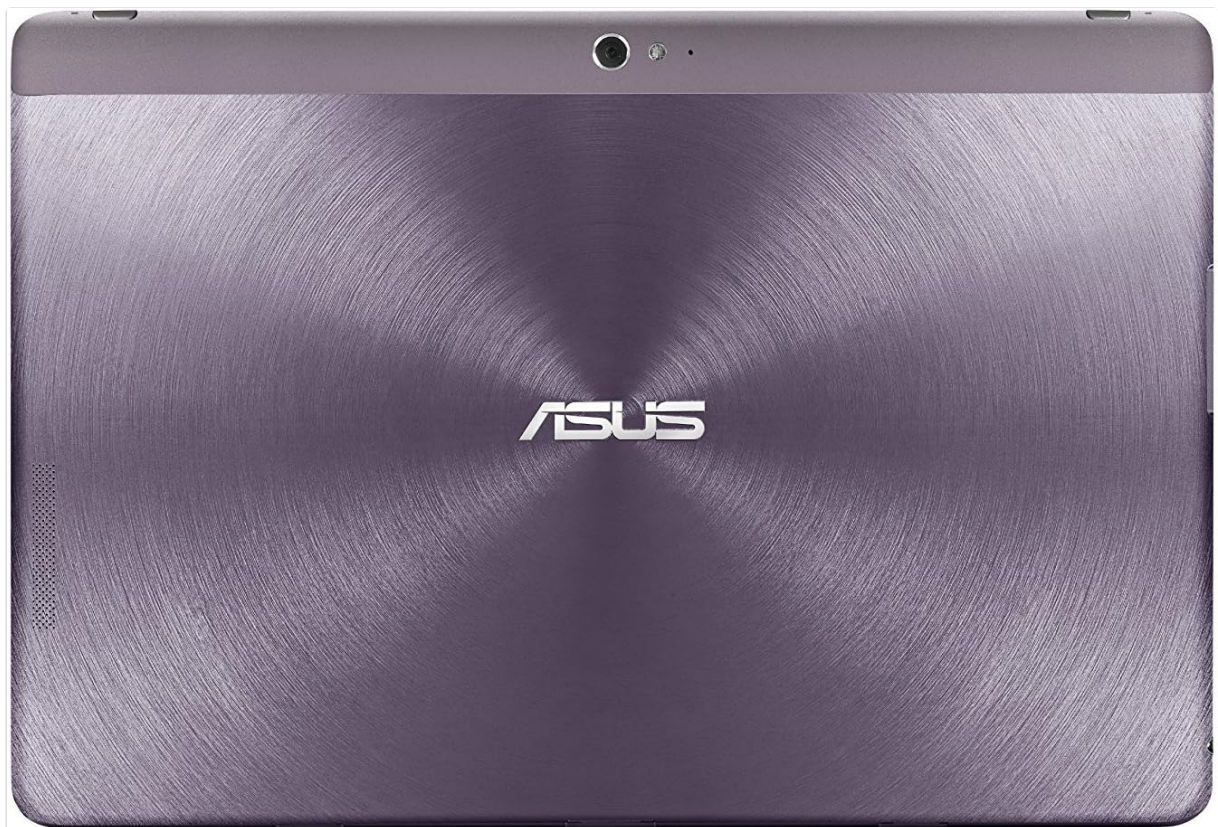
Figure 4.1: Rear view of the tablet, highlighting the distinctive metallic spun finish and the placement of the 8MP rear camera.
