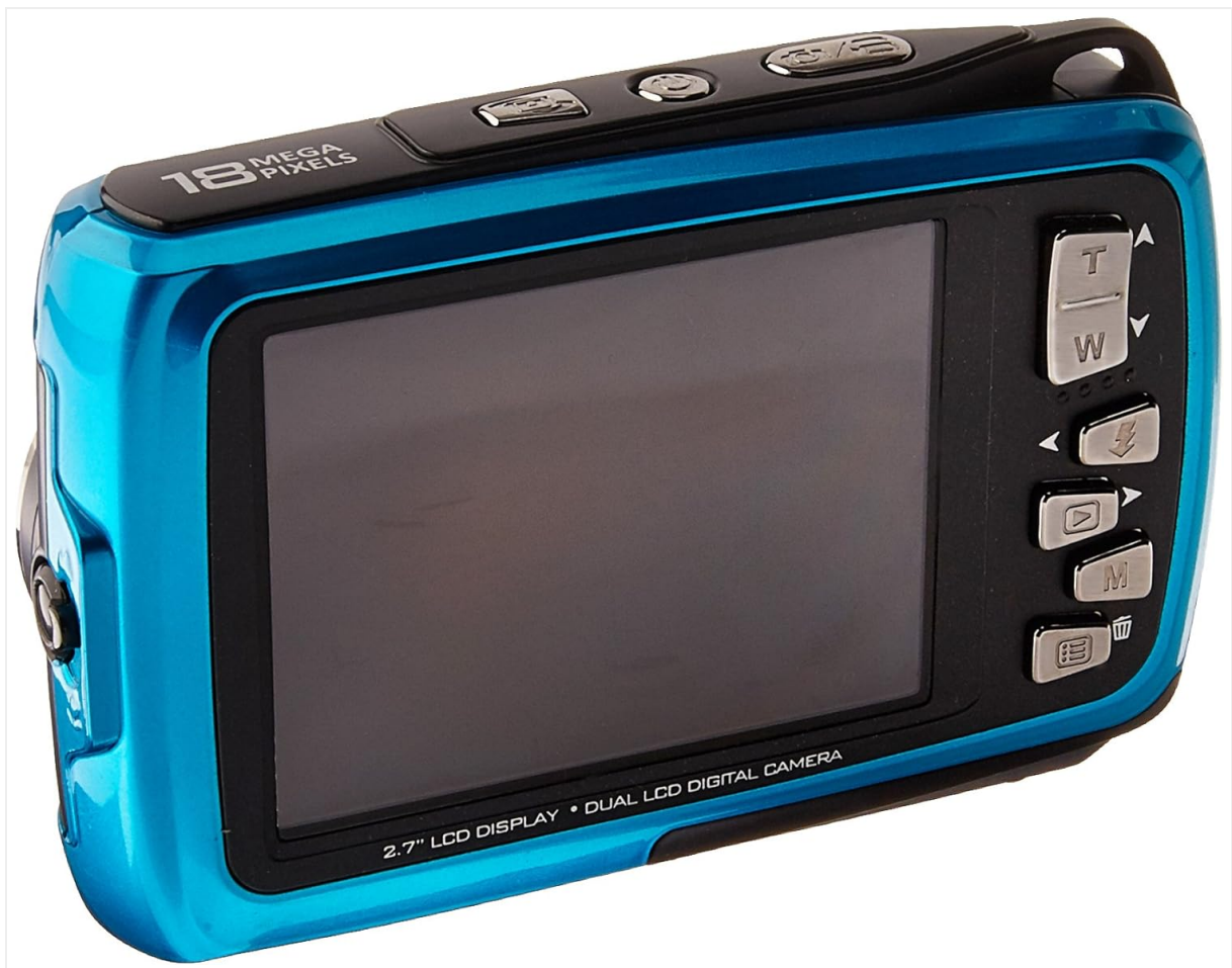
Figure 2: Rear view of the SVP Aqua5500 camera, highlighting the 2.7" LCD display and control buttons. Key controls include the power button, shutter button, zoom controls (T/W), mode button (M), and playback button.
