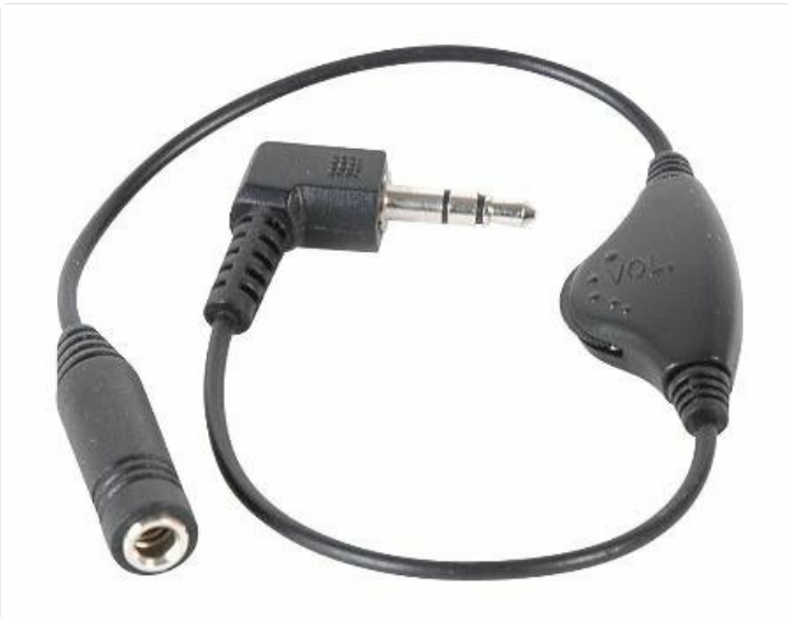
Image: The Stellar Labs Inline Volume Control showing its male 3.5mm plug on the right, the female 3.5mm jack on the left, and the central volume dial. This illustrates how the unit connects between an audio source and headphones.
