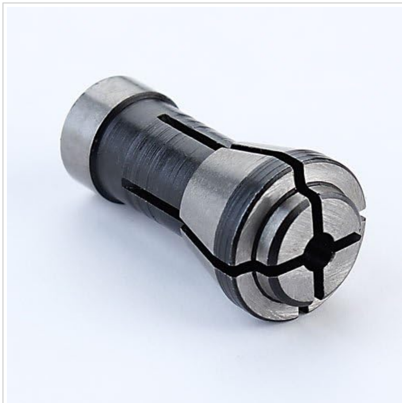
Figure 1: The Grex 1/8" Collet. This image displays the metal collet, which is a precision-machined cylindrical component. One end features a solid base, while the other end is split into four segments, designed to flex and securely grip a tool shank when tightened within a collet nut. The collet has a dark, textured body with polished metal ends.
