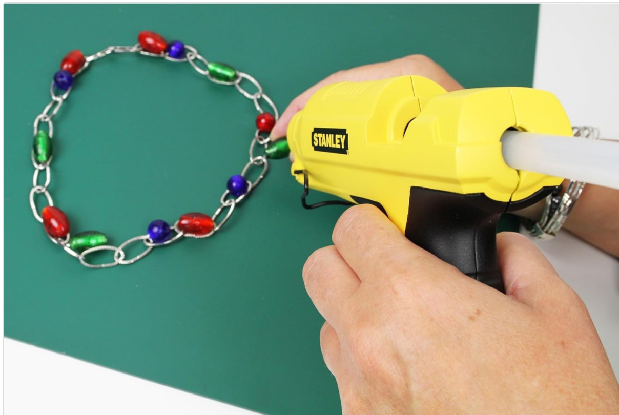
Image: A person holding the Stanley STH6-70417 glue gun, demonstrating how to hold it during use. A glue stick is visible at the rear of the tool.
