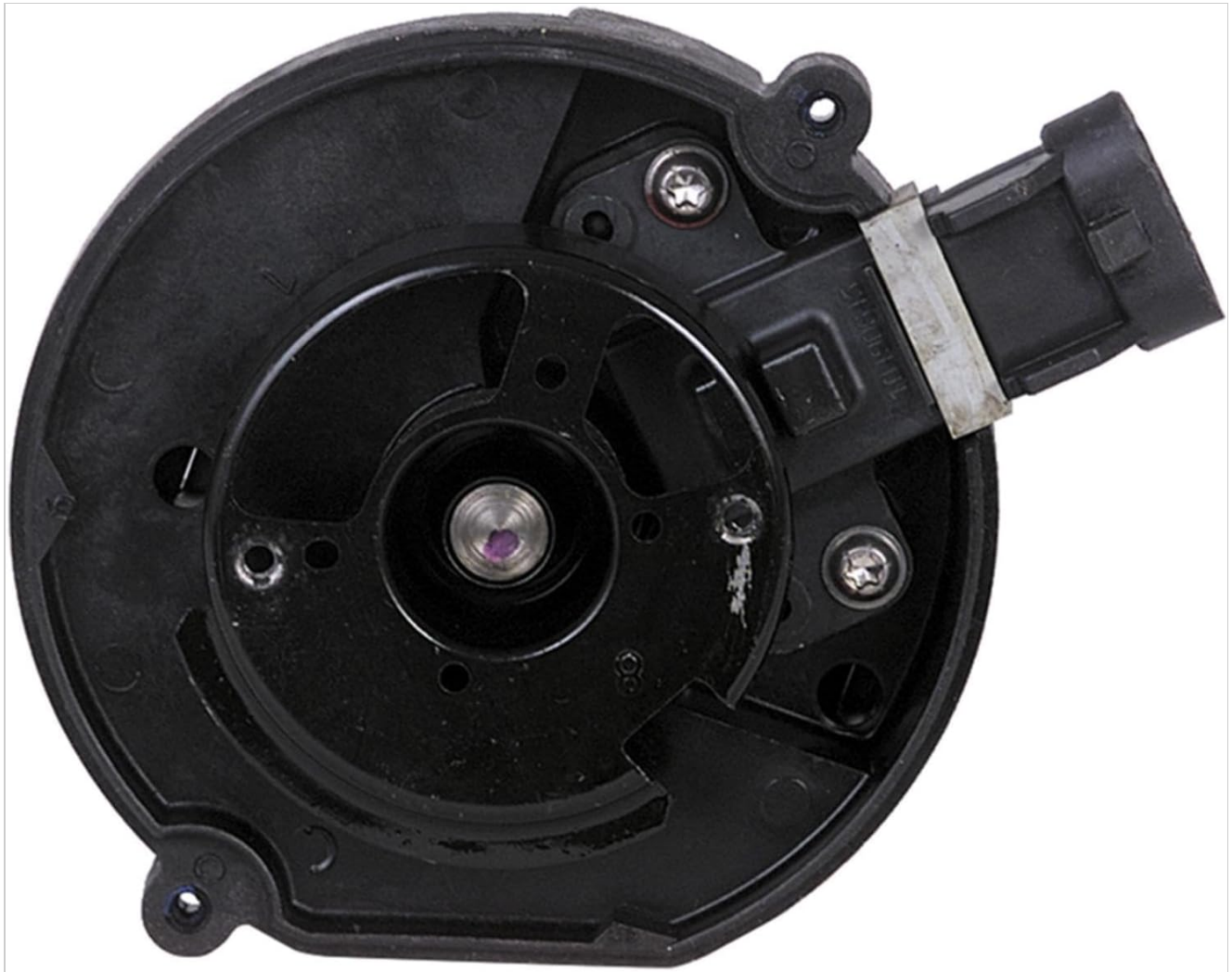
Figure 4: Top view of the ignition distributor, showing the cap mounting points.
