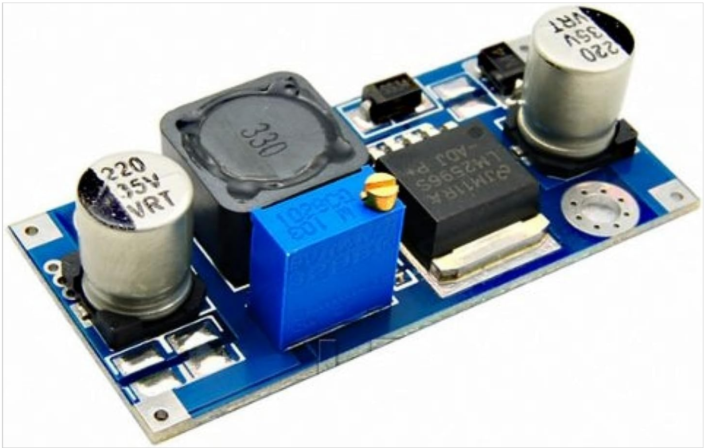
Figure 2.1: Top view of the LM2596 DC-DC Buck Converter module, showing the input/output terminals, potentiometer, inductor, and capacitors.
