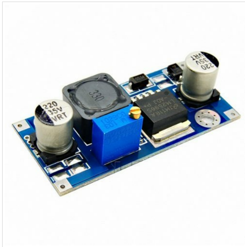
Image: RioRand LM2596 DC-DC Buck Converter Module. This image shows the compact design of the module with its input/output terminals and the blue potentiometer for voltage adjustment.
