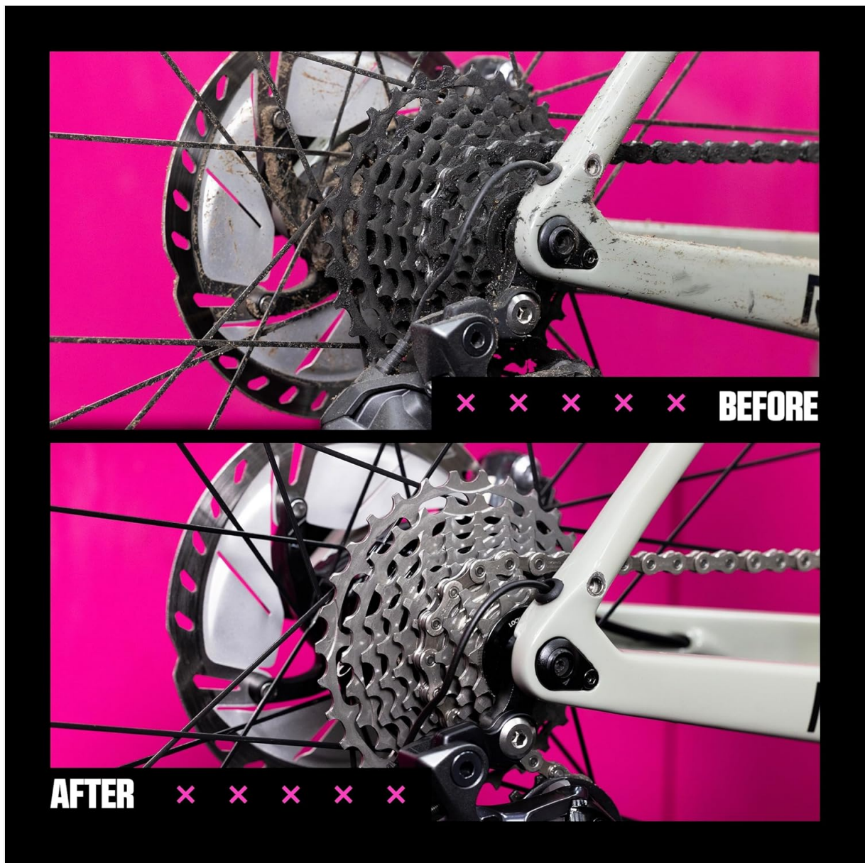
Image 4: Before and after cleaning results on a bicycle cassette.
