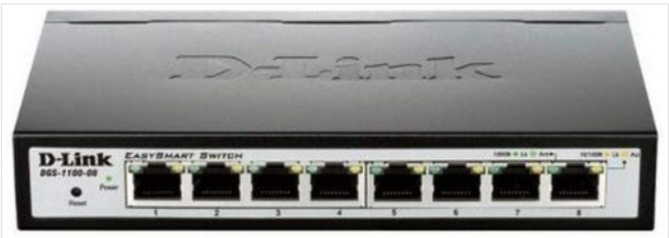
Figure 4.2: Front view of the D-Link DGS-1100-08 switch, clearly displaying the eight Gigabit Ethernet ports labeled 1 through 8, along with the Power LED and Reset button.
