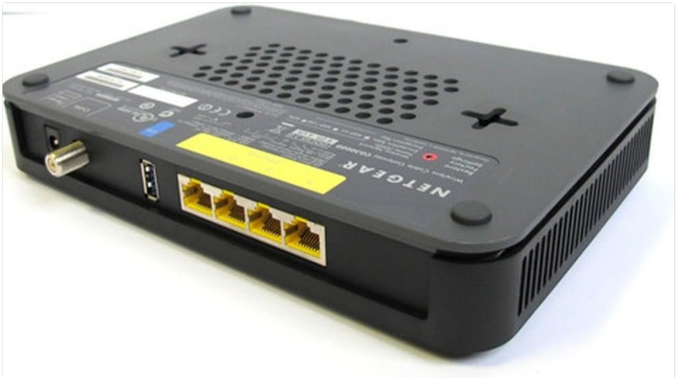
Figure 2: Back view of the NETGEAR CG3000D-100NAS Cable Modem Router, showing Ethernet LAN ports, USB port, coaxial cable connector, power adapter input, and power on/off button.
