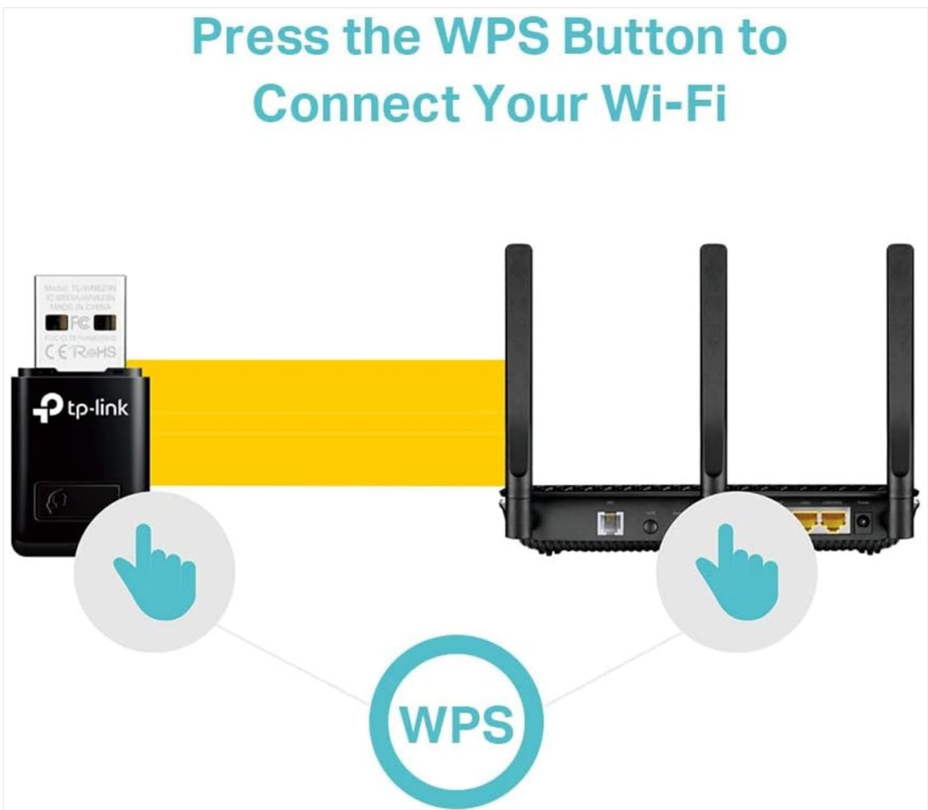
Figure 3.2: WPS Connection with Router
