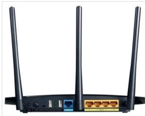
Figure 3.2: Rear view of the TL-WDR4300 router, showing the power input, On/Off button, USB ports, WAN port, LAN ports, and WPS/Reset button.
