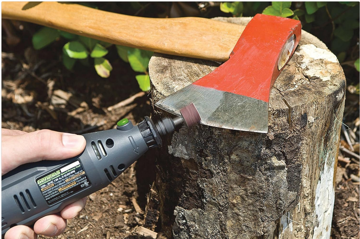
Image 4: The rotary tool being used to sharpen an axe blade, showcasing its utility for sharpening various tools.
