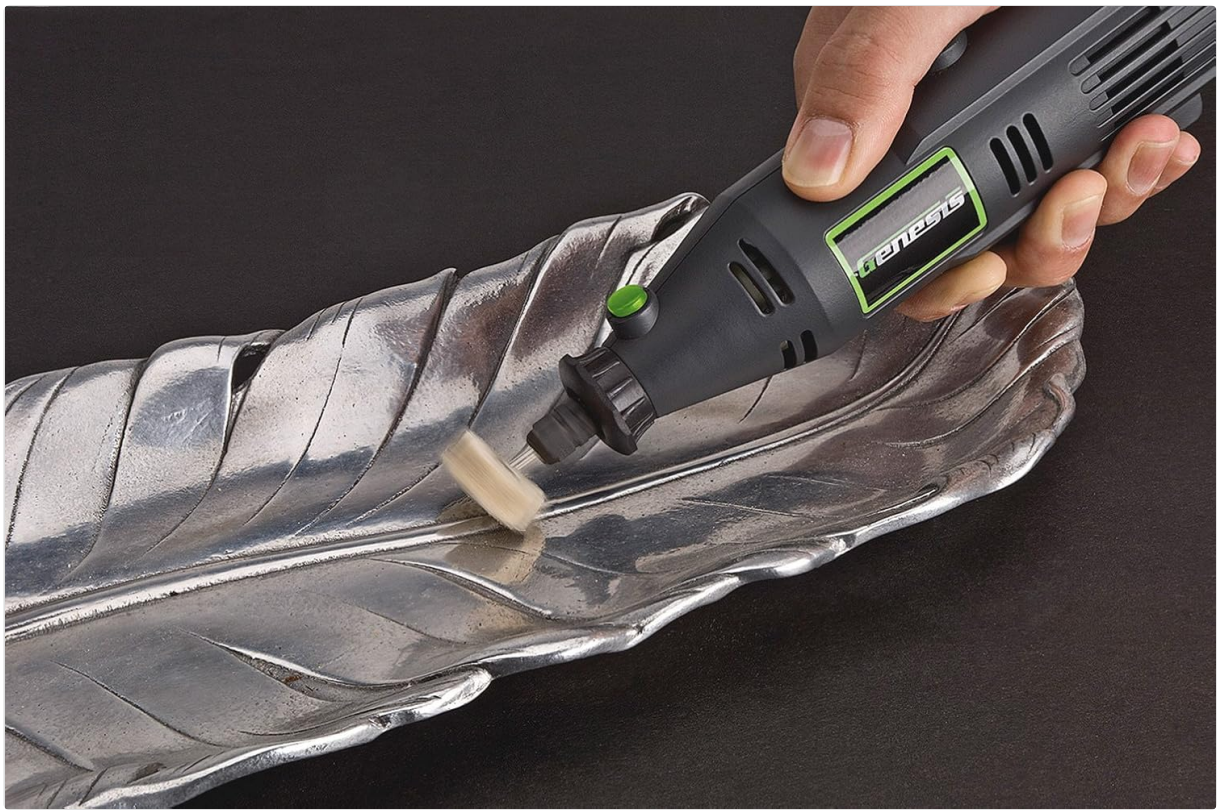
Image 3: A user polishing a decorative metal tray with the rotary tool, highlighting its use for finishing and buffing tasks.
