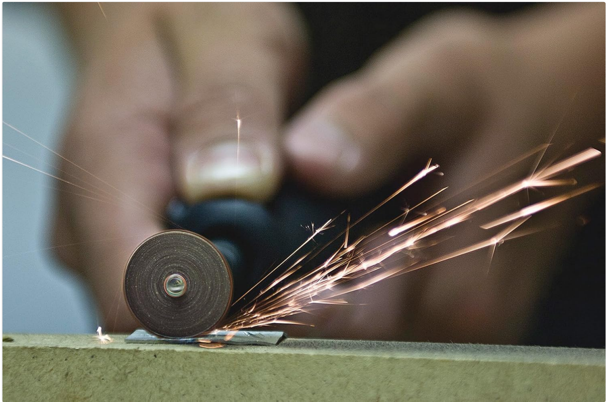
Image 2: The rotary tool in use for cutting a small metal piece, demonstrating its capability for precise material removal.
