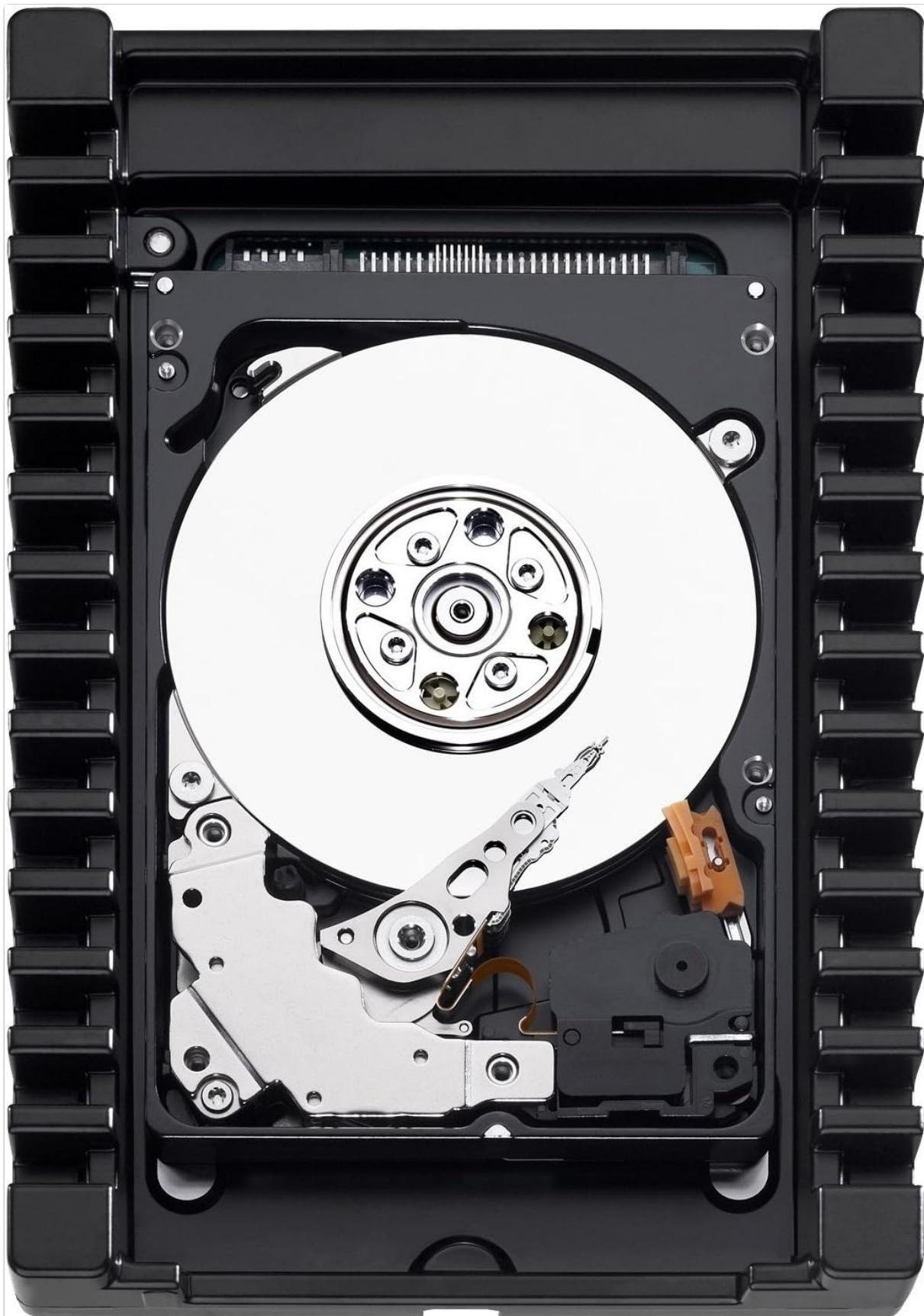
This image displays the internal components of the WD VelociRaptor hard drive, including the shiny data platters, the delicate read/write head assembly, and the robust black heat sink enclosure designed for optimal cooling. The SATA data and power connectors are visible at the top edge.
