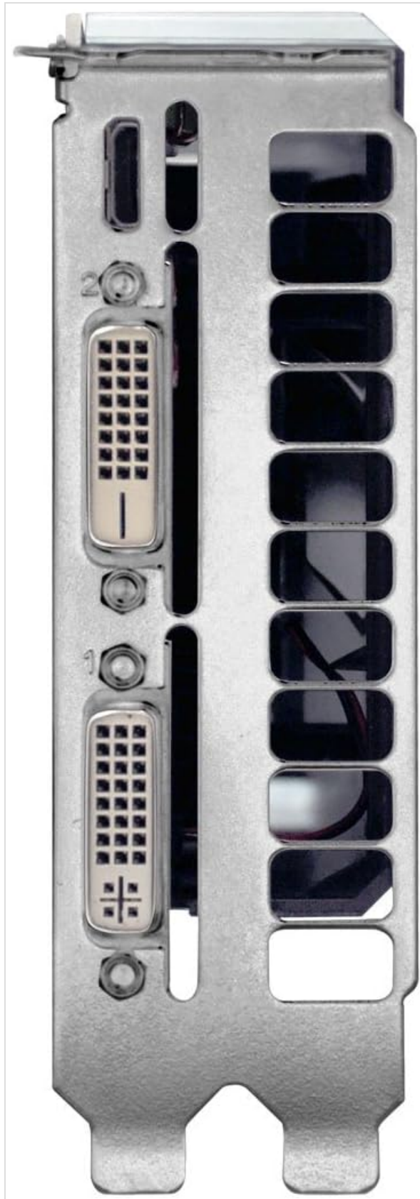
Figure 3.1: Display output ports on the EVGA GeForce GT 640 graphics card, including two DVI ports and one mini-HDMI port.
