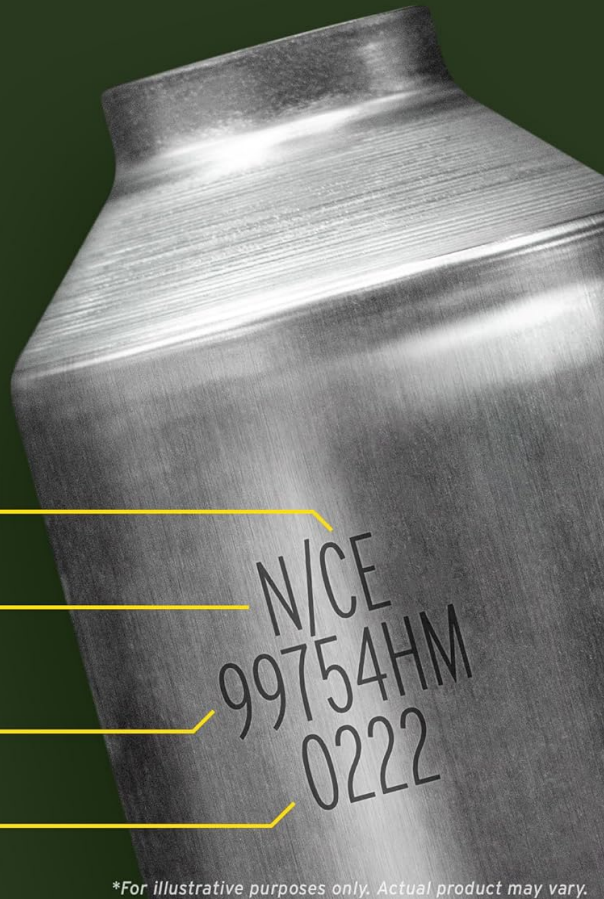
Figure 4: Detailed view of the markings on a catalytic converter, illustrating how to identify an EPA compliant unit with codes for manufacturer, new converter status, part number application, and manufacturing date.
