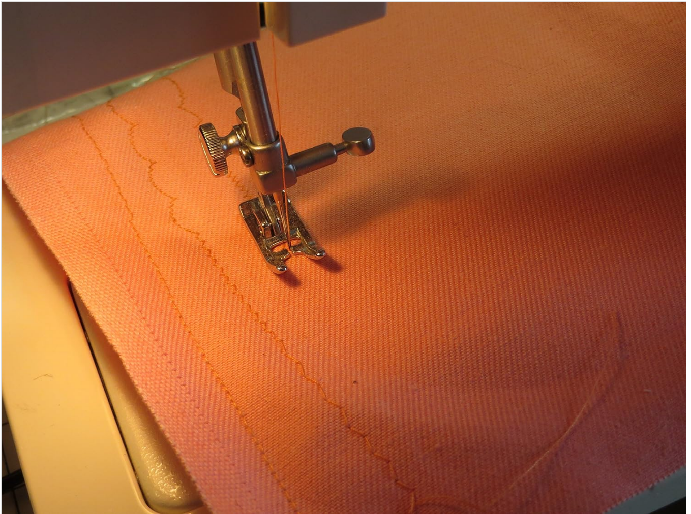
Figure 5: Needle and Presser Foot in Action. This detailed shot focuses on the needle and presser foot as they sew through fabric, demonstrating the machine's operation during stitching.
