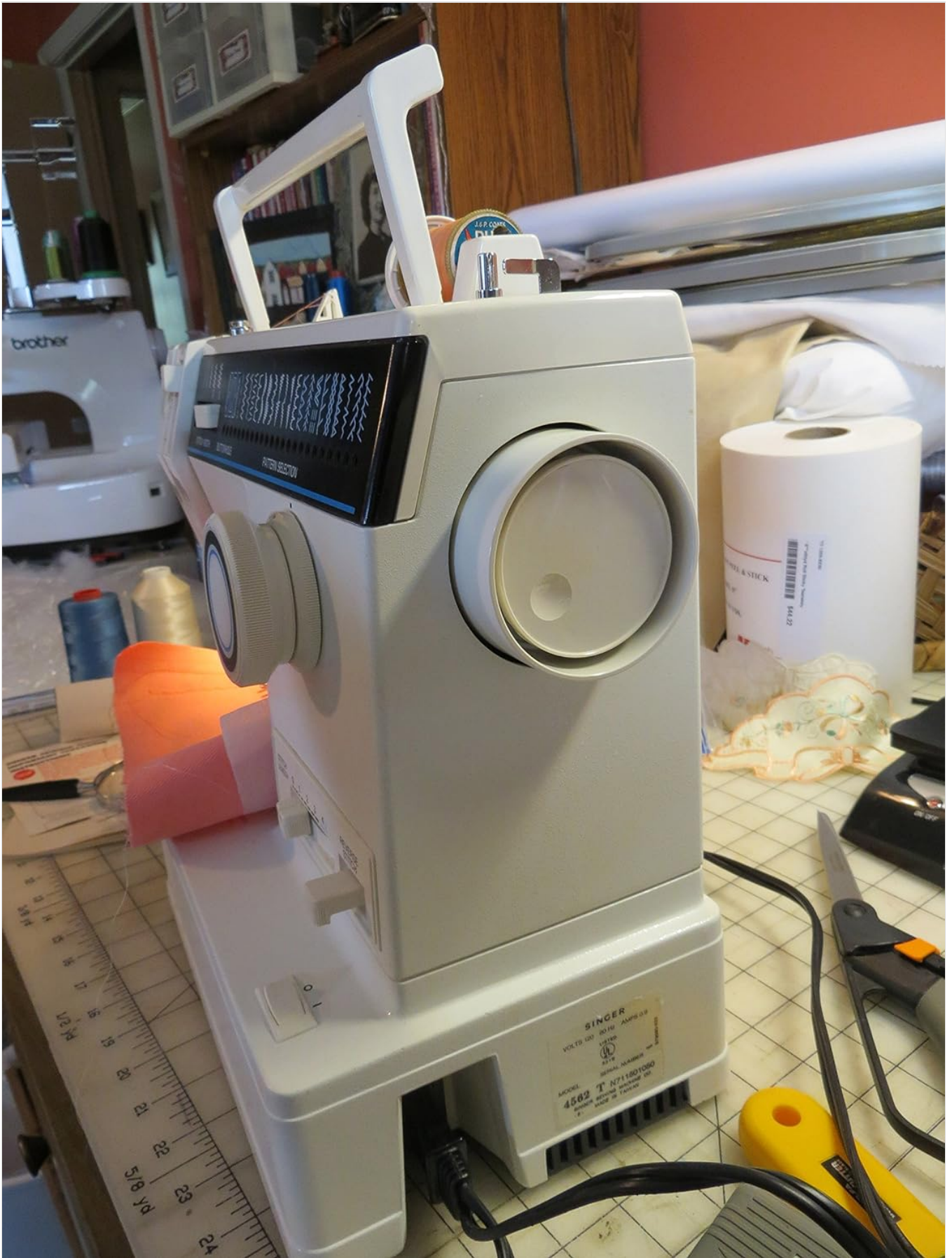
Figure 2: Side View and Power Connection. This view shows the right side of the sewing machine, including the handwheel, power input, and foot pedal connection. The model number "4562" is visible on the machine's base.
