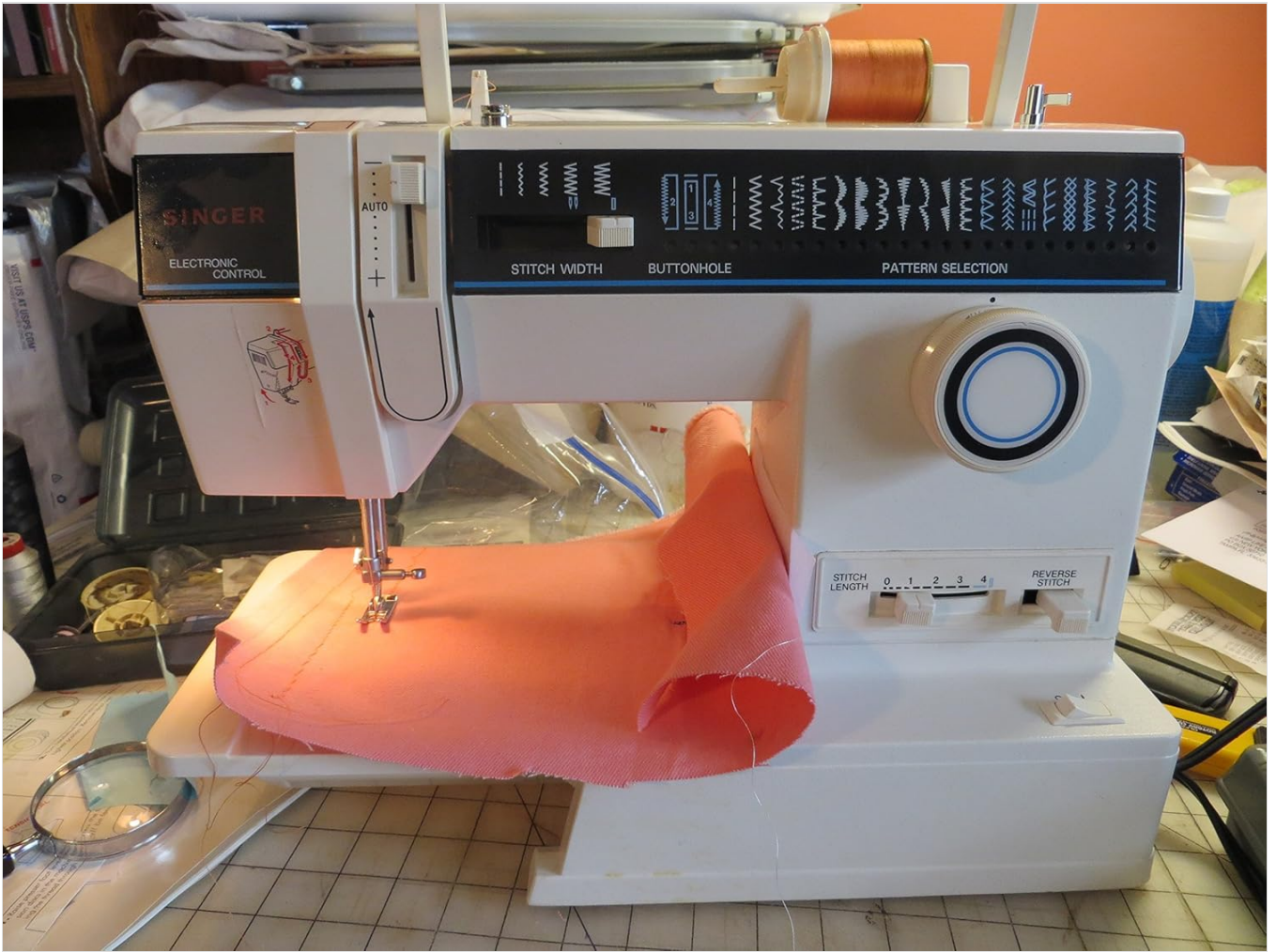
Figure 1: Front View of SINGER Model 4562. This image displays the front of the sewing machine, highlighting the needle area, presser foot, stitch selection panel, and the free arm feature with fabric in place. Key controls like stitch width and buttonhole settings are visible on the top panel.
